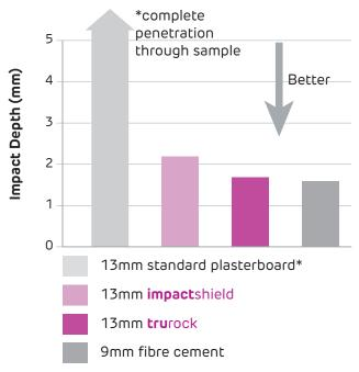
**FIGURE 22 Small Hard Body Impact Testing** 2.4m drop height
