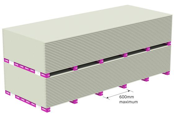
FIGURE 1 Correct Plasterboard Storage
