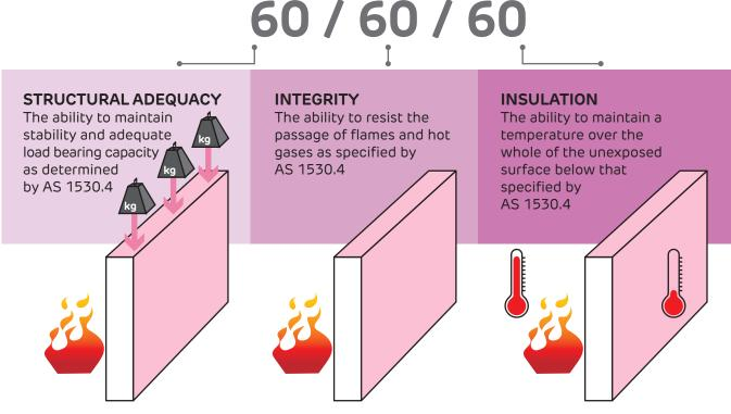
FIGURE 10 Fire Resistance Level
