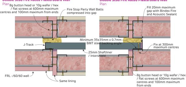
FIGURE 37 Interhome High-Rise Wall Transition to Double Stud Fire Rated Plasterboard Wall
