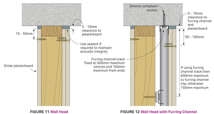
FIGURE 12 Wall Head with Furring Channel Section
