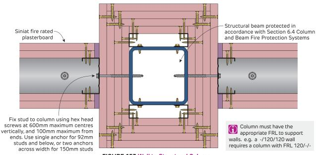
FIGURE 153 Wall to Structural Column
