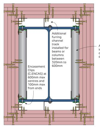
For corner gaps up to 3mm, fill with either Bindex Fire and Acoustic sealant or Mastabase jointing compound. Fill any other gaps with Bindex sealant to maintain integrity.
