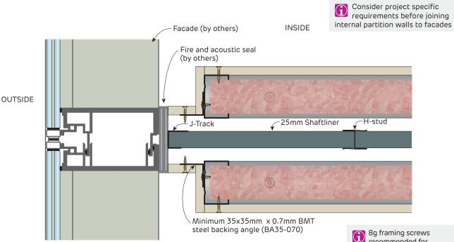
FIGURE 48 Interhome High-Rise Wall Transition to Curtain Wall Mullion  $\mathsf{Plan}$
