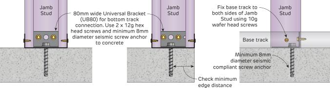
FIGURE 26a Base Connection BC6 for Prefabricated Door Frames Section
