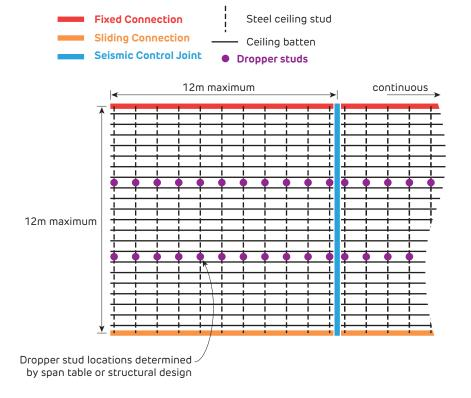
FIGURE 38 Stud Ceiling Type A3 - Fixed / Sliding
