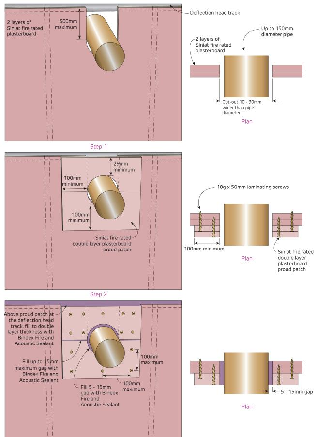
Step 3 FIGURE 221 Proud patch around metal pipe penetration near deflection head track
