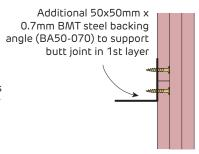
FIGURE 14 Laminated Vertical Shaft Butt Joint in 1st Layer
