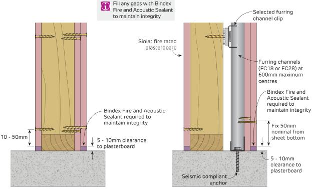
FIGURE 17 Wall Base Section
