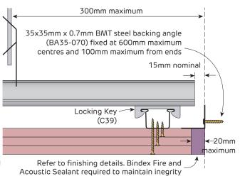
FIGURE 55 Top Cross Rail End Detail
