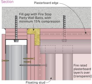
FIGURE 147 Sliding Wall End To Plasterboard
