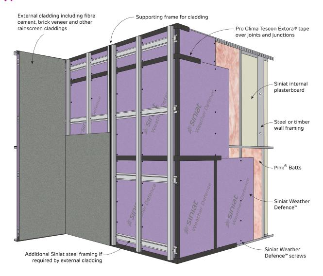
**FIGURE 1 Typical Weather Defence Installation**Perspective
