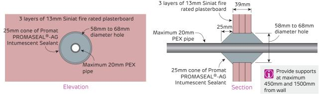
FIGURE 31 20mm PEX Pipes
