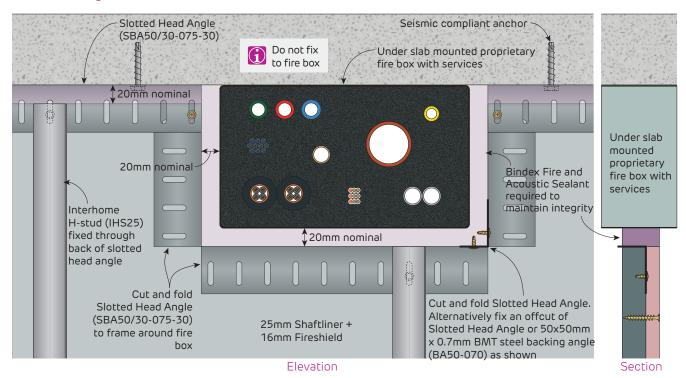
FIGURE 74 Under Slab Mounted Fire Box Detail through Central Fire Barrier
