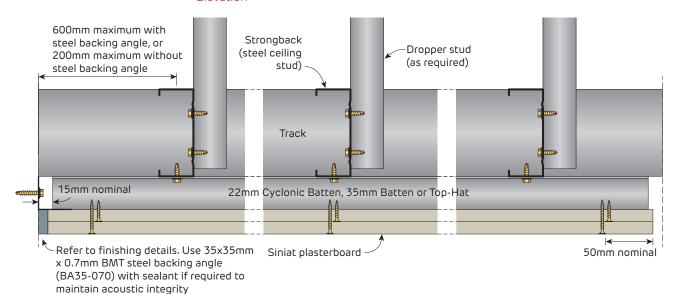
**SECTION G-G Ceiling Edge** Section **SECTION G-G Ceiling Stud Detail** Section
