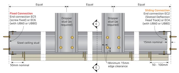
FIGURE 35 Stud Ceiling Type A2 - Fixed / Sliding Elevation
