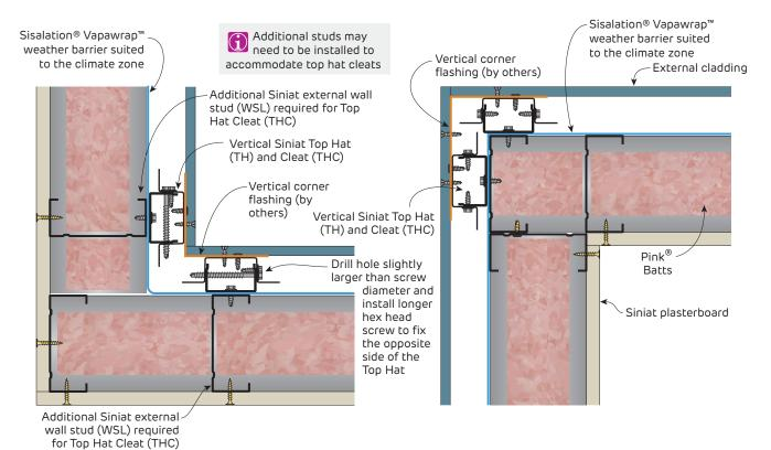
FIGURE 10 External Steel Stud Wall Internal Corner
