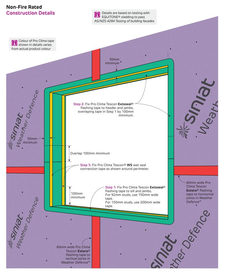
**FIGURE 36 Alternative Flashing Tape Around Openings**Perspective
