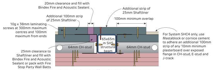
FIGURE 7 Shaft Wall Ceiling with SHS Structural Beam
