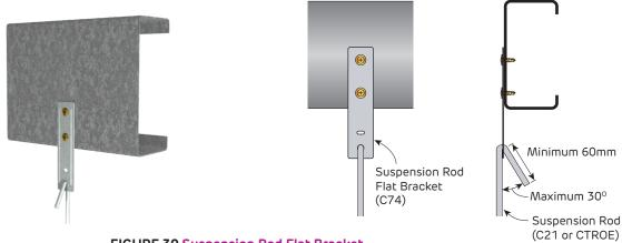
FIGURE 30 Suspension Rod Flat Bracket Perspective and Sections
