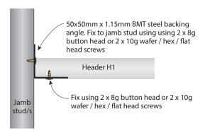
FIGURE 24b Alternative Header H1 Connection 'A-2' Elevation
