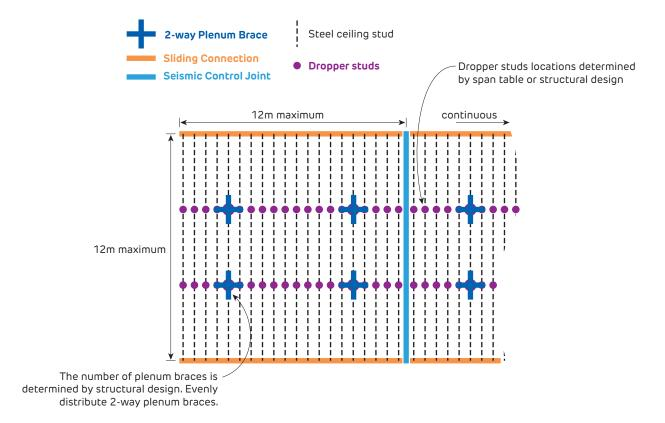
FIGURE 49 Stud Ceiling Type C1 - 2-way Plenum Braced Plan
