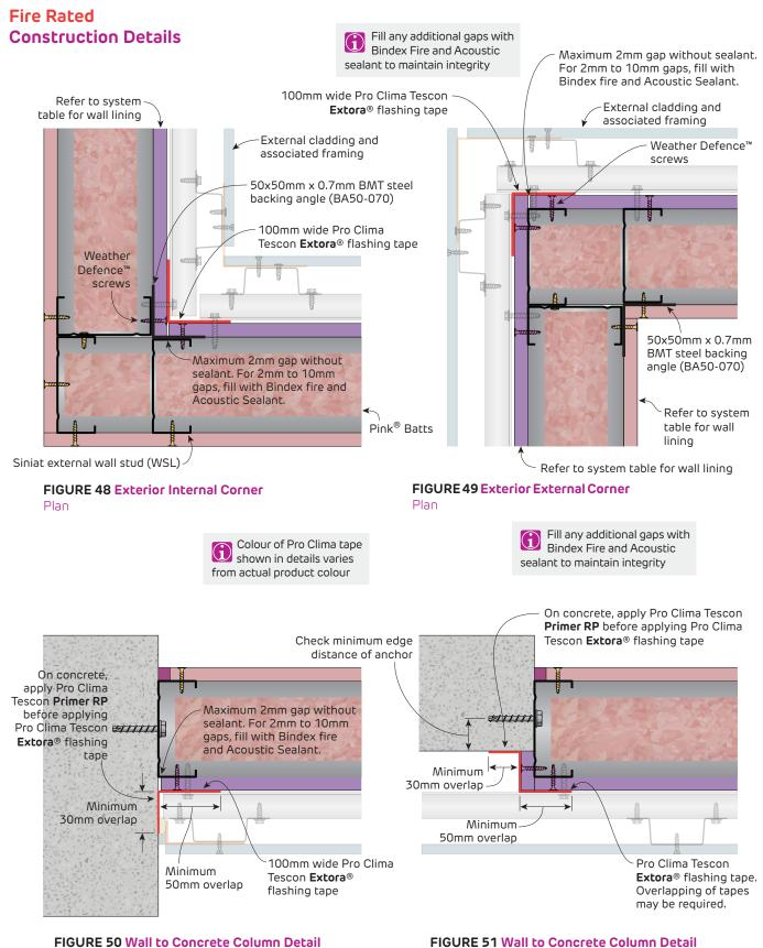
FIGURE 51 Wall to Concrete Column Detail
