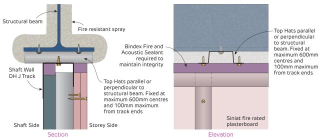
FIGURE 36 Internal Wall to Structural Beam
