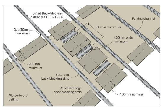
FIGURE 2 Placement of Back-Blocking Batten and Back-Blocking Strips for Recessed and Butt Joints
