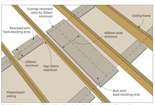
FIGURE 1 Placement of Back-Blocking Strips For Recessed and Butt Joints
