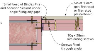
FIGURE 16 Laminated Vertical Shaft Transition to Steel Framed Partition Wall
