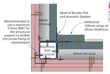
FIGURE 14 Detail using SHS Beam with 64mm CH-Studs
