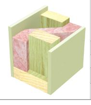
Stud Depth Wall Width Sound Insulation (mm) Rw (Rw + Ctr) (mm) Pink<sup>®</sup> Batts Pink® Batts Polyester Report insulation Wall R1.5 Wall R2.0 R1.5 Day Design 70 on 3094-45 110 36 (29) 43 (34) 45 (36) 43 (34) 90mm plate Note: Impact 90 on Sound 140 37 (32) 45 (37) 46 (38) 44 (37) 120mm plate Resistant
