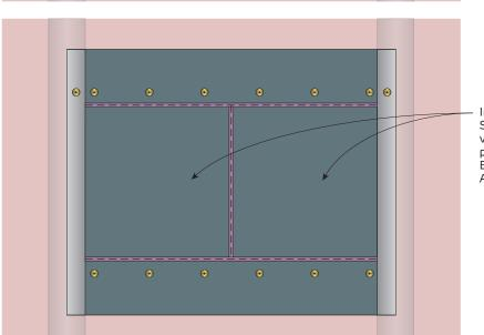
Insert two pieces of Shaftliner panel into void and seal 5 - 20mm perimeter gaps with Bindex Fire and Acoustic Sealant
