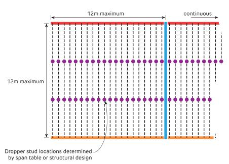
FIGURE 34 Stud Ceiling Type A2 - Fixed / Sliding
