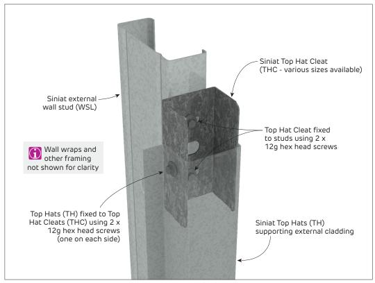
FIGURE 4 Top Hat Cleat over External Steel Stud Wall
