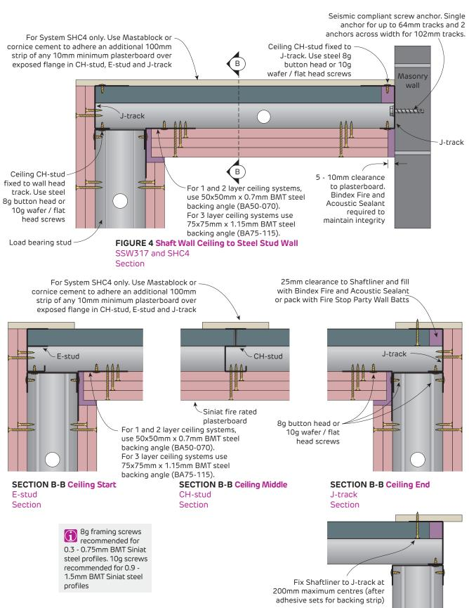
SECTION B-B Construction of Ceiling End J-track
