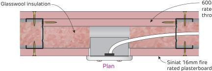
600mm high baffle using 16mm fire rated plasterboard fixed using 2 screws through steel studs on each side
