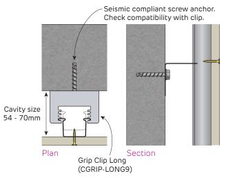
**FIGURE 12 Grip Clip Long**With 9mm hole suitable for 6mm Screw Anchor
