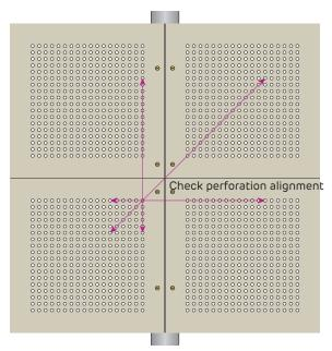
**FIGURE 17 Perforation Alignment** Plan
