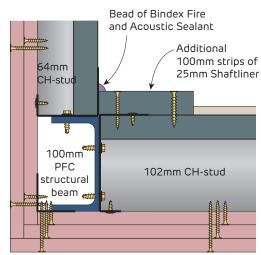
FIGURE 18 Detail using PFC Beam with 64 and 102mm CH-Studs
