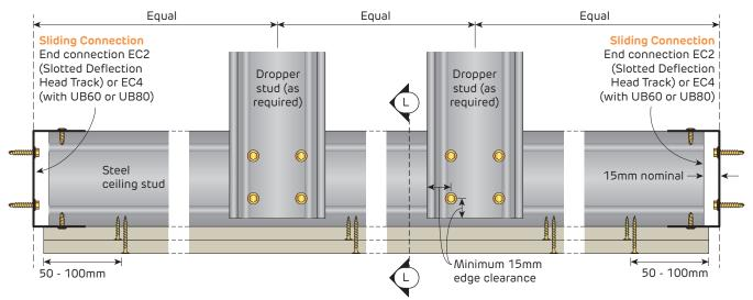
FIGURE 50 Stud Ceiling Type C1 - 2-way Plenum Braced
