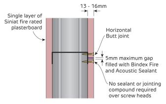
FIGURE 231 Horizontal Joints in Single Layer Wall Systems
