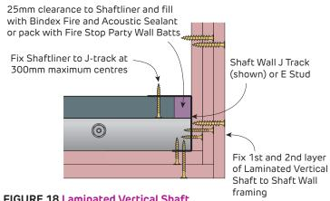
FIGURE 18 Laminated Vertical Shaft Corner Transition to Shaft Wall Plan view
