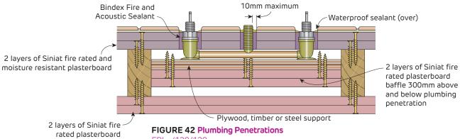
FRL -/120/120 Fire rated double layer system - Plan
