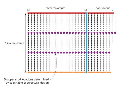
FIGURE 42 Stud Ceiling Type A4 - Fixed / Sliding
