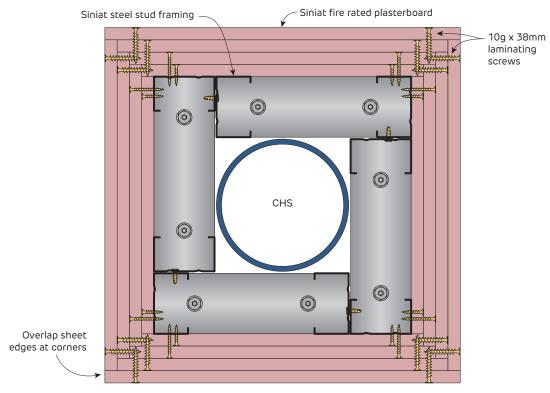
**FIGURE 11 4 Sided Protection for CHS** Plan
