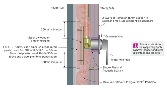
FIGURE 47 Mixer Tap or Tapset Penetration with 102mm CH-stud
