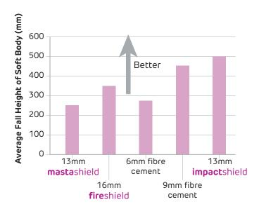
FIGURE 19 Soft Body Impact Testing
