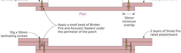
Fill any gaps with Bindex Fire and Acoustic sealant to maintain integrity
