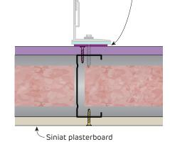
FIGURE 16 Weather Defence **Installation with Top Hats** Plan
