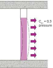
Case 4: Internal Wall  $C_{p,i net} = 0.3$
