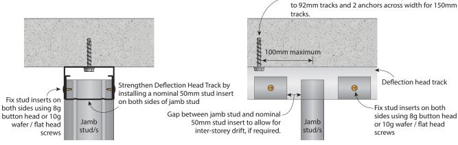
FIGURE 16b Head Track Connection HC6 Section
