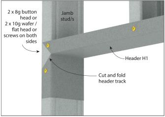
FIGURE 23a Header H1 Connection 'cut and fold' Perspective
