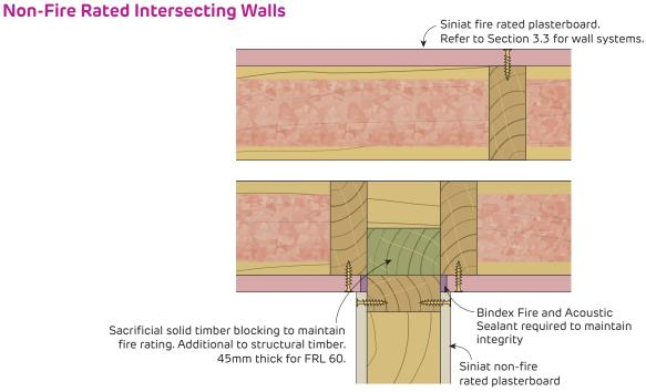
FIGURE 12 Separating Wall with Non-Fire Rated Intersecting Wall
