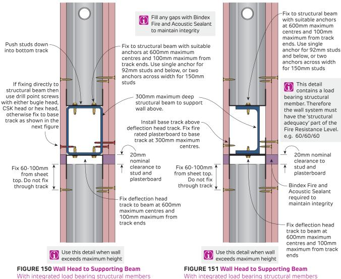
With integrated load bearing structural members Section
