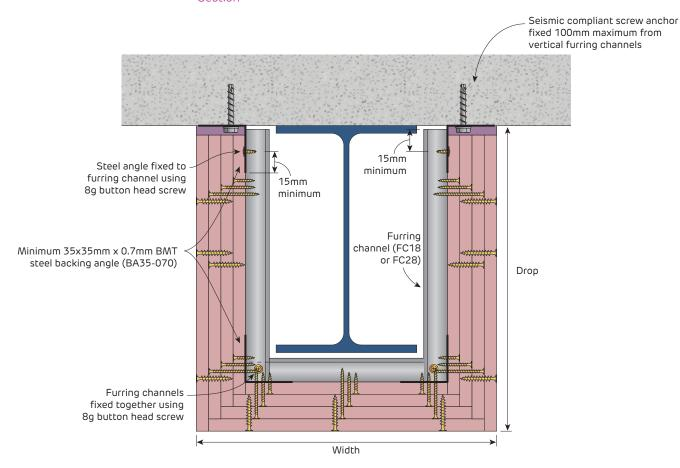
**FIGURE 8 U-Shaped Bulkhead** Section
