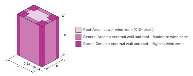
FIGURE 3 Typical Simplified Wind Zones on a Building
