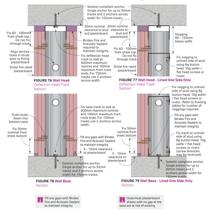
8g framing screws recommended for 0.3 - 0.75mm BMT Siniat steel profiles. 10g screws recommended for 1.15 -1.5mm BMT Siniat steel profiles
