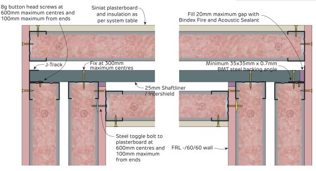
FIGURE 31 Interhome High-Rise Wall Connection to Fire Rated Plasterboard Wall Plan
