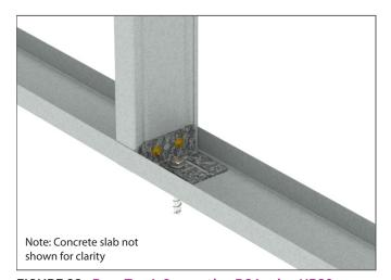
**FIGURE 22a Base Track Connection BC4 using UB80** Heavy Duty Connection for 92mm and 150mm studs Perspective
