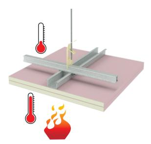
FIGURE 11 Resistance to Incipient Spread of Fire
