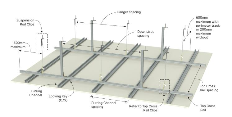
FIGURE 6 Suspended Ceiling Frame with Downstruts
