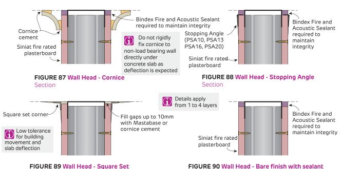
FIGURE 90 Wall Head - Bare finish with sealant
