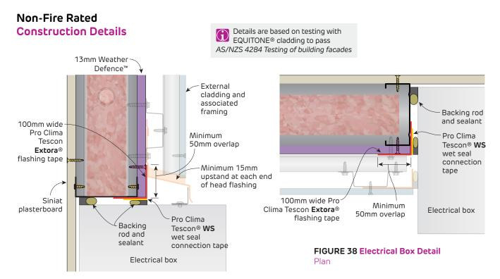
FIGURE 37 Electrical Box Detail
