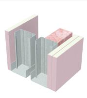
1 layer of 16mm fireshield or multishield or trurock
