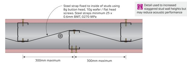
FIGURE 17 Strap Nogging for Staggered Stud Walls Plan
