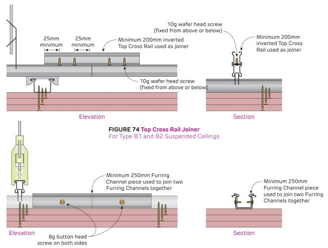
**FIGURE 75 Furring Channel Joiner**For Type B1 and B2 Suspended Ceilings
