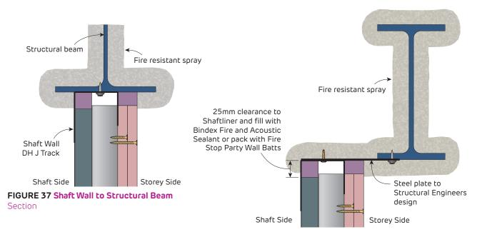
**FIGURE 38 Shaft Wall to Structural Beam** Section
