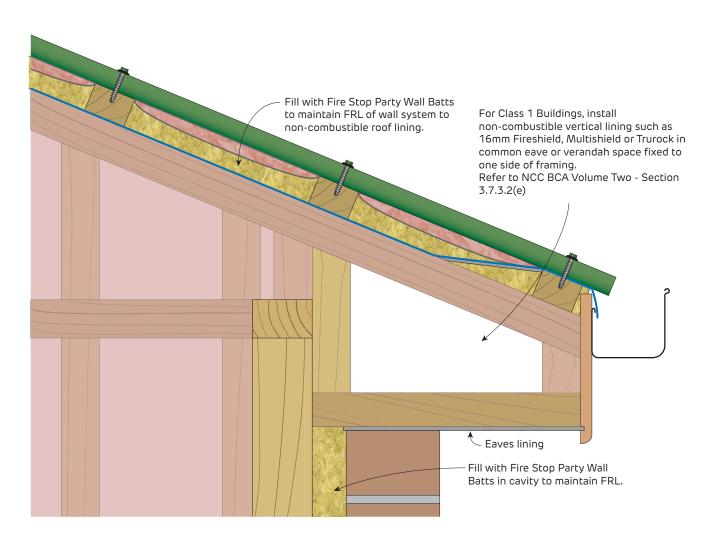
FIGURE 11 Separating Wall Over Eaves Lining
