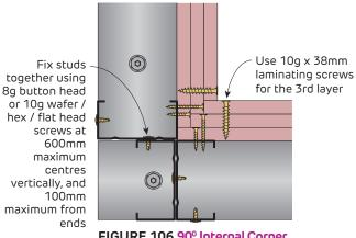
Up to 3 layers of Siniat fire rated plasterboard 0 50x50mm x 0.7mm BMT steel backing angle (BA50-070) Seismic compliant anchor
