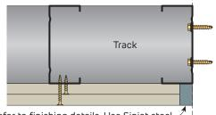
Refer to finishing details. Use Siniat steel of stud or steel backing angle with sealant if required to maintain acoustic integrity
