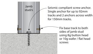
FIGURE 19b Base Track Connection BC3
