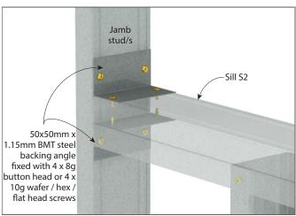
FIGURE 28a Sill S2 Connection '2A-2'
