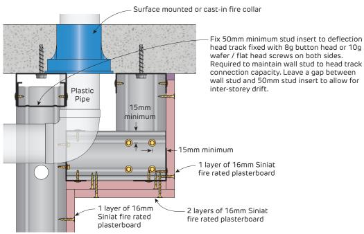
FIGURE 228 Bulkhead for Plastic Pipe clash
