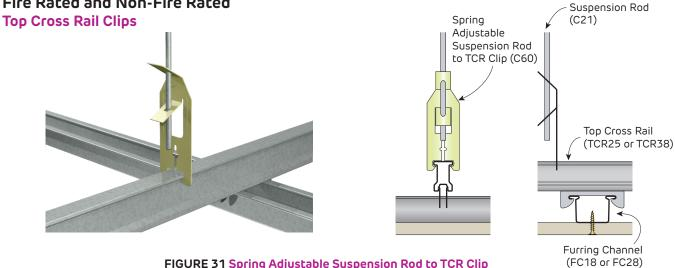
FIGURE 31 Spring Adjustable Suspension Rod to TCR Clip Perspective and Sections
