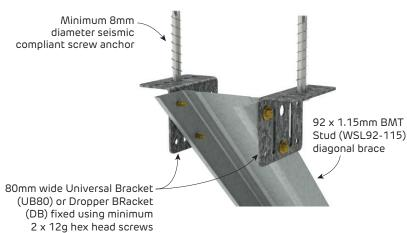
**FIGURE 82 Alternative Diagonal Brace Soffit Connection**Perspective
