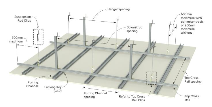
**FIGURE 6 Suspended Ceiling Frame with Downstruts**Perspective
