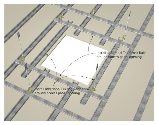
**FIGURE 15 Creason Access Panel Framing**Perspective
