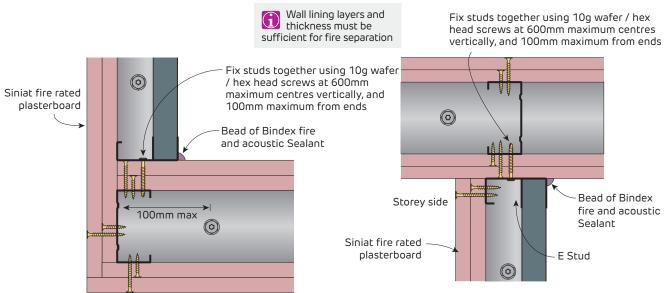
FIGURE 31 Shaft Wall to Internal Partition Corner Plan
