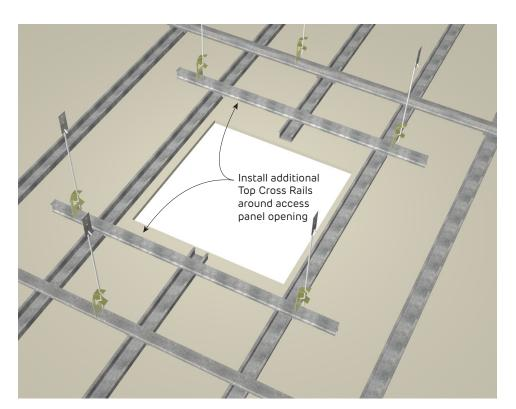
**FIGURE 14 Creason Access Panel Framing**Perspective
