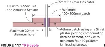
Maintains FRL of ceiling under floor/roof systems Patch above ceiling lining Valid for 1 layer systems only - Section
