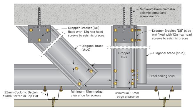
FIGURE 57 2-way Plenum Brace Elevation
