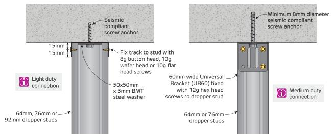
FIGURE 13 Concrete Soffit Connection SC1
