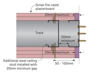
**SECTION B-B Alternative Ceiling Edge** Section
