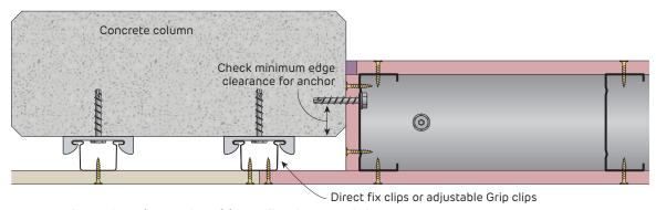
FIGURE 156 Fire rated Partition Wall to Concrete Column
