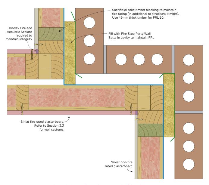
FIGURE 14 Separating Wall to External Brick Wall
