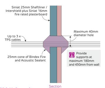
FIGURE 66 TPS Cable Penetration
