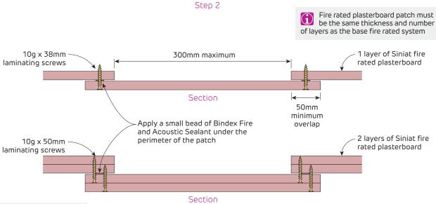
Fill any gaps with Bindex Fire and Acoustic sealant to maintain integrity
