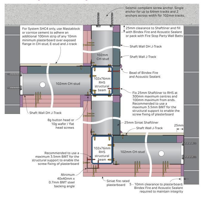
**FIGURE 26** Shaft Wall Ceilings and Bulkhead using RHS Structural Columns and Beams SHW2 and SHC4
