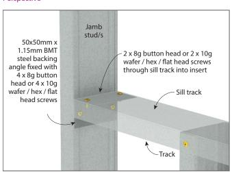
FIGURE 27a Alternative Sill S1 Connection 'A-2' Perspective
