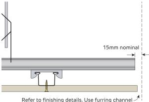
track or steel backing angle with sealant if required to maintain acoustic integrity
