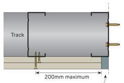
Refer to finishing details. Use perimeter steel stud or 35x35mm x 0.7mm BMT steel backing angle (BA35-070) with sealant if required to maintain acoustic integrity
