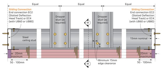
FIGURE 51 Stud Ceiling Type C1 - 2-way Plenum Braced Elevation
