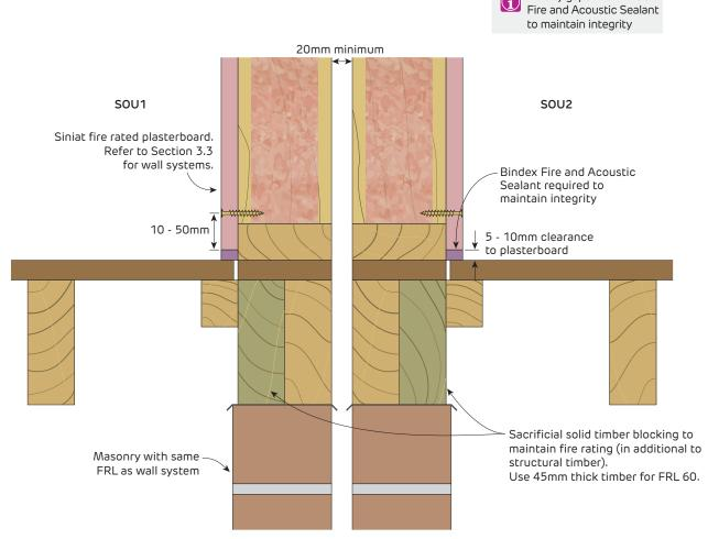
**FIGURE 2 Separating Wall with Suspended Ground Floor** FRL 60/60/60 Section
