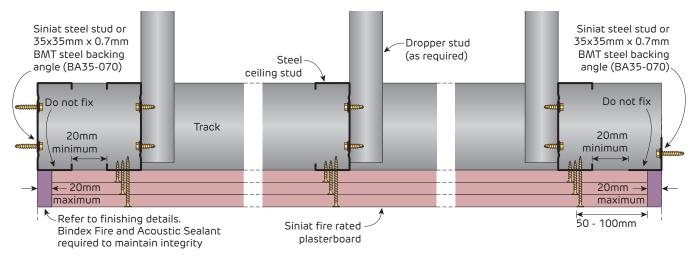
SECTION M-M Ceiling Edge Section **SECTION M-M Ceiling Stud Detail** Section
