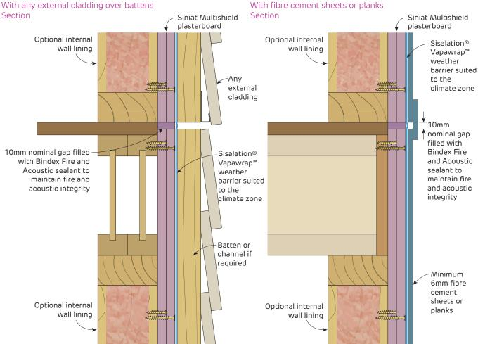
FIGURE 10 External Timber Wall with Suspended Floor
