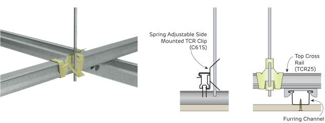
FIGURE 32 Spring Adjustable Side Mounted TCR Clip Perspective and Sections
