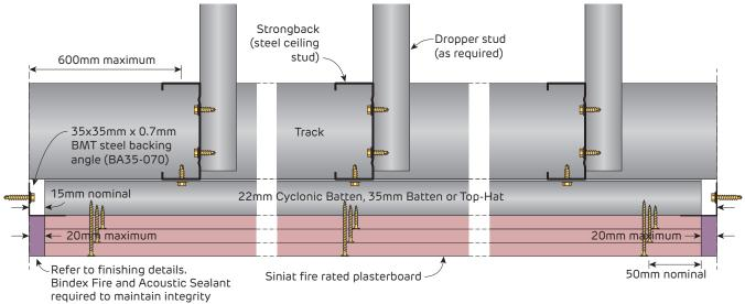
SECTION O-O Ceiling Edge Section **SECTION O-O Ceiling Stud Detail** Section
