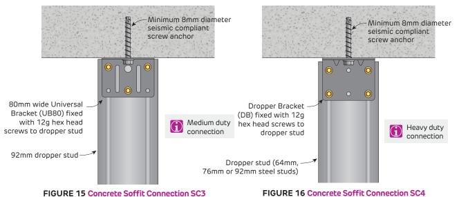
FIGURE 15 Concrete Soffit Connection SC3
