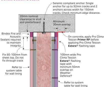
Details are based on testing with EQUITONE® cladding to pass AS/NZS 4284 Testing of building facades.
