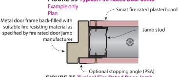
FIGURE 35 Typical Fire Rated Door Jamb
