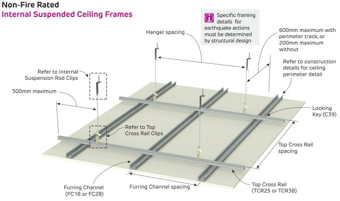
**FIGURE 5 Suspended Ceiling Frame**Perspective
