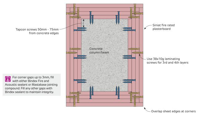
FIGURE 13 4 Sided Protection Concrete Column/Beam Plan
