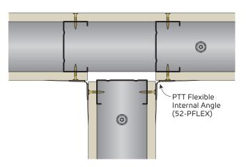
**FIGURE 65 Sliding Intersecting Wall** Plan
