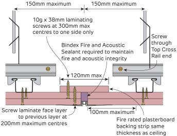
FIGURE 100 Seismic Control Joint
