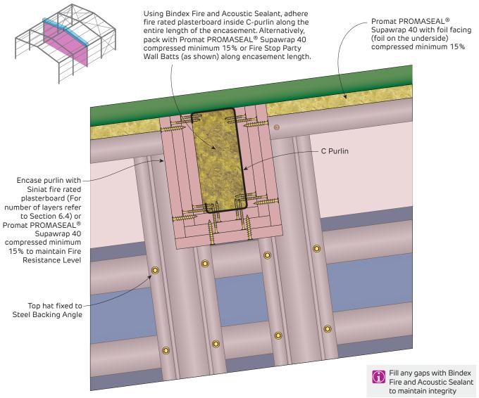
FIGURE 3 Wall Head Detail for C Purlin Up to FRL 120/120/120
