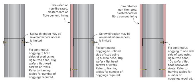
FIGURE 3 Continuous Nogging Track
