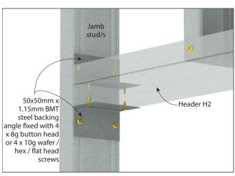
8g framing screws recommended for 0.3 - 0.75mm BMT Siniat steel profiles.10g screws recommended for 1.15 - 1.5mm BMT Siniat steel profiles
