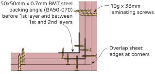
**FIGURE 10 Laminated Vertical Shaft External Corner** Plan view
