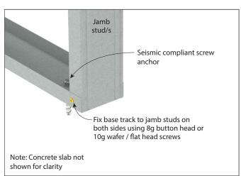
FIGURE 19a Base Track Connection BC3 - Doorway Perspective
