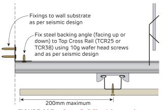
FIGURE 66 Top Cross Rail Fixed Connection
