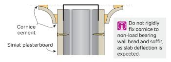
**FIGURE 49 Wall Head - Cornice** Section
