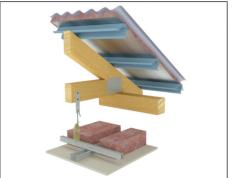
[Lateral restraint of truss bottom chord must be considered, ie: bottom chord ties and steelbrace]
