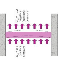
Case 3: Internal Wall C<sub>p.inet</sub> = 0.4
