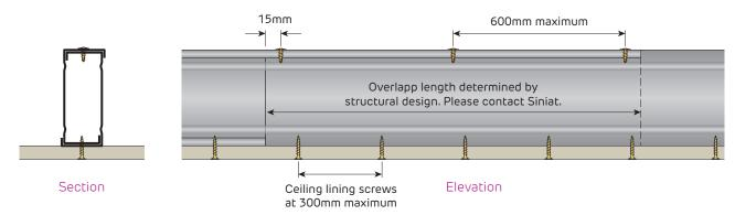
FIGURE 58 Splicing Steel Ceiling Studs via Overlap Method
