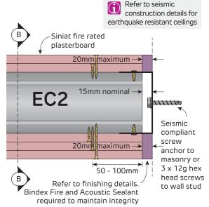
FIGURE 10 Sliding Connection EC2 Slotted Deflection Head Track Section
