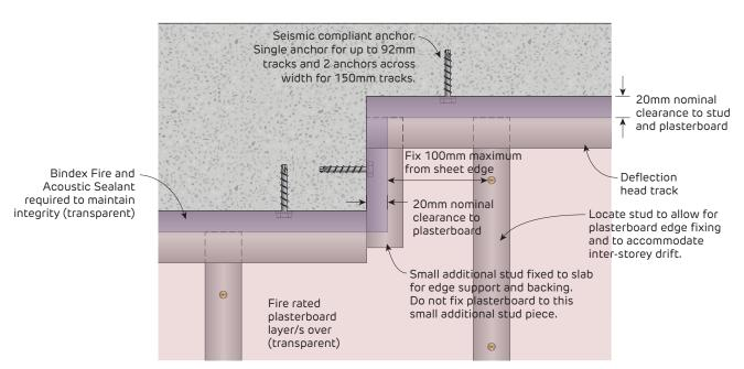
FIGURE 139 Step in Concrete Slab with 20mm allowance for Inter-Storey Drift Elevation
