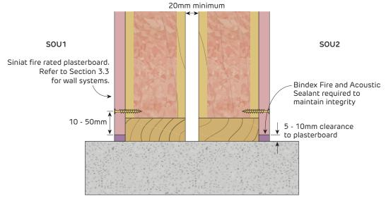
**FIGURE 1 Separating Wall Base to Slab** FRL 60/60/60 Section
