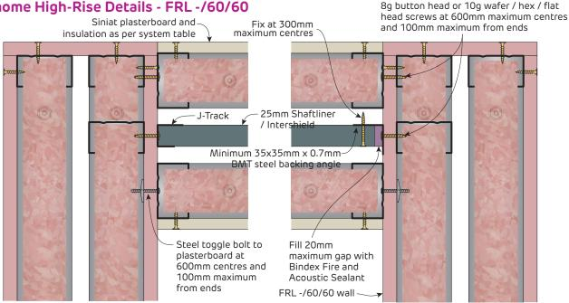
FIGURE 29 Interhome High-Rise Wall Connection to Fire Rated Plasterboard Wall Plan
