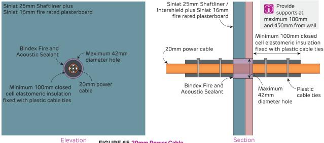
FIGURE 65 20mm Power Cable FRL -/60/60
