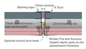
FIGURE 28 Shaft Wall Control Joint
