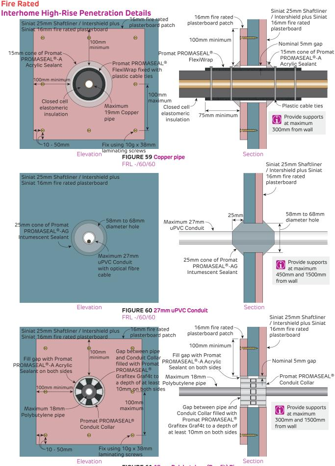
FIGURE 61 18mm Polybutylene (Pro-fit) Pipes
