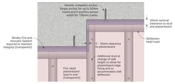
FIGURE 138 Step in Concrete Slab Elevation
