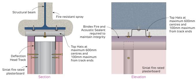
FIGURE 154 Internal Wall to Structural Beam
