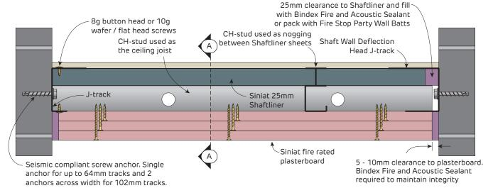
FIGURE 1 Shaft Wall Ceiling to Masonry Wall Section
