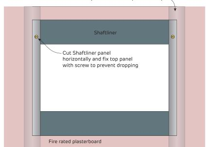
Cut flanges off ends of minimum 51mm wall track centred wall track and centre between CH Studs
