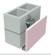
This system is designed to upgrade the FRL of the masonry wall
