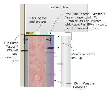
FIGURE 39 Electrical Box Detail
