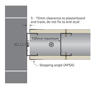
FIGURE 64 Sliding Wall End To Masonry
