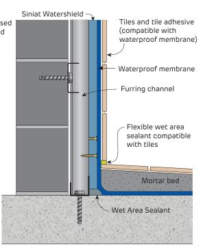
**FIGURE 11 Shower over Masonry Wall** Class 3 membrane shown - Section
