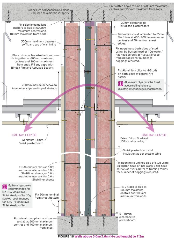
Slotted Steel Angle above Shaftliner Section
