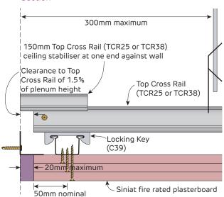
FIGURE 87 Top Cross Rail Free Edges
