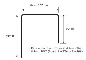
**FIGURE 4 Shaft Wall Deflection Head J Track** Section
