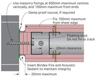
FIGURE 148 Sliding Wall End To Masonry Plan
