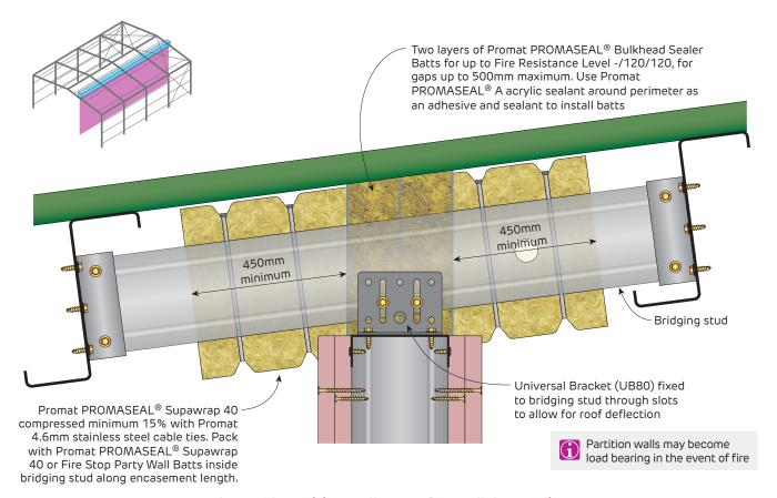
FIGURE 12 Partition Wall to Roof - Parallel to Purlins
