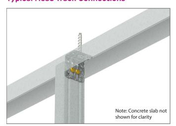
**FIGURE 17a Head Track Connection HC4 using UB60** Heavy Duty Connection for 64mm and 76mm studs Perspective
