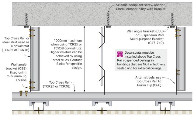
FIGURE 12 Downstrut Section
