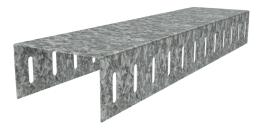
**FIGURE 10 Slotted Deflection Head Track** 92 x 1.15mm BMT Perspective
