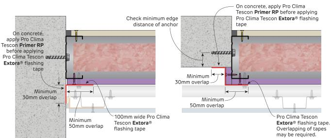
**FIGURE 21 Wall to Concrete Column Detail** Plan
