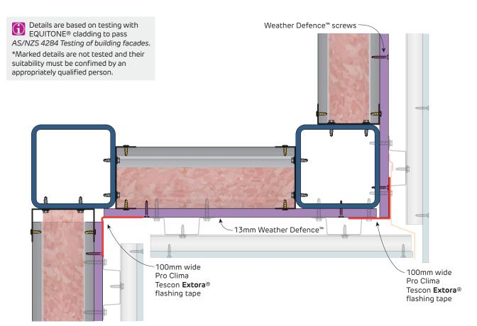
FIGURE 30 Soffit Junction
