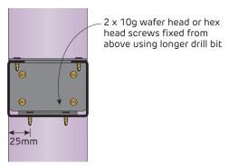
FIGURE 18a Header to Jamb Stud Connection for Prefabricated Door Frames Section
