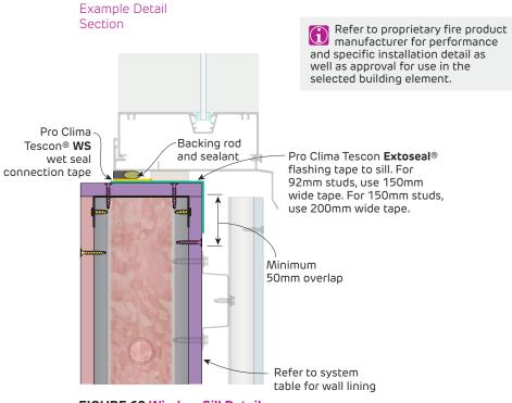
FIGURE 60 Window Sill Detail
