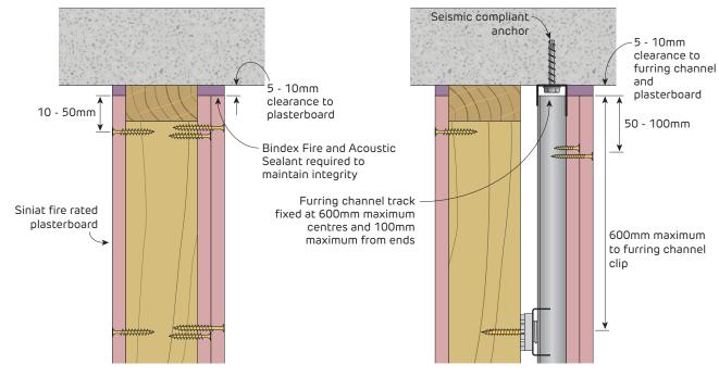
FIGURE 15 Wall Head Section
