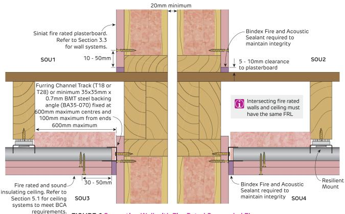
FIGURE 6 Separating Wall with Fire Rated Suspended Floor  $\mathsf{FRL}\,60/60/60$
