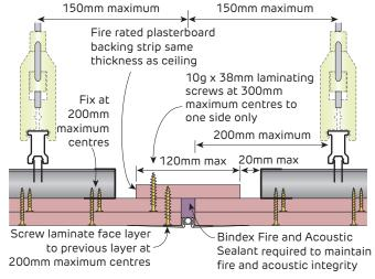
FIGURE 101 Seismic Control Joint
