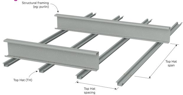
FIGURE 1 Top Hat Span and Spacing
