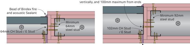
Bindex Fire and Acoustic Sealantrequired to maintain integrity
