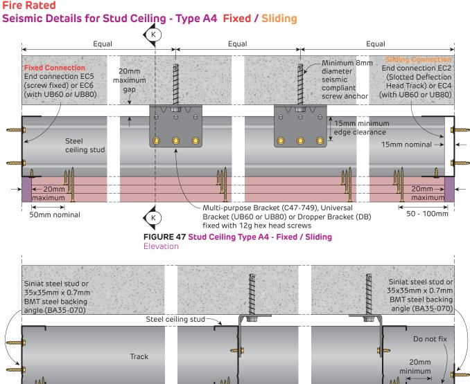
Refer to finishing details. Bindex Fire and Acoustic Sealant required to maintain integrity **SECTION K-K Ceiling Edge**
