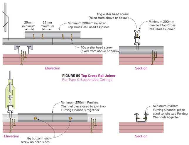
**FIGURE 90 Furring Channel Joiner**For Type C Suspended Ceilings
