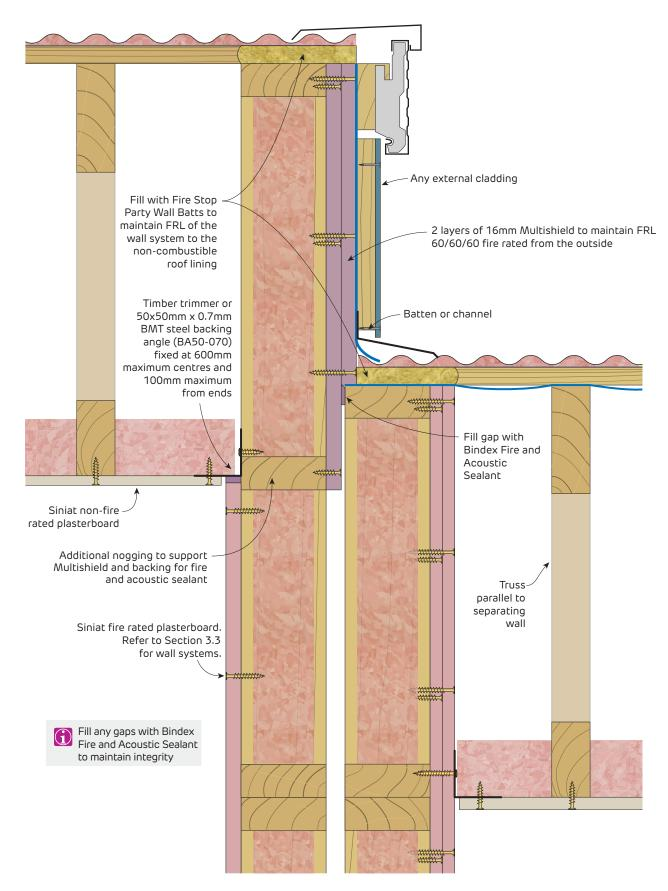
FIGURE 10 Separating Wall with External Wall Above  $\mathsf{FRL}\,60/60/60$
