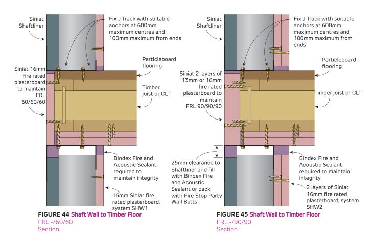
50mm minimum overlap Particleboard Siniat 2 layers of flooring 13mm or 16mm fire Timber joist or CLT rated plasterboard to maintain FRL 90/90/90 Fix at 400mm maximum centres and 100mm maximum from 50mm minimum overlap **Bindex Fire and Acoustic** Sealant required to maintain integrity
