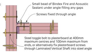
**FIGURE 8 Laminated Vertical Shaft T Intersection**Plan view
