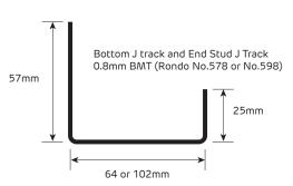
FIGURE 3 Shaft Wall J Track Section
