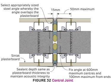
FIGURE 31 Control Joint
