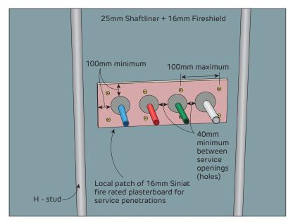
**FIGURE 51 Local Patch for Penetrations Through Central Fire Barrier** With example service penetrations Perspective
