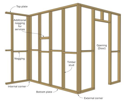
FIGURE 1 Internal Timber Frame Wall Layout
