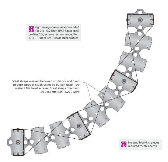
**FIGURE 18 Strap Nogging for Curved Stud Walls** Plan
