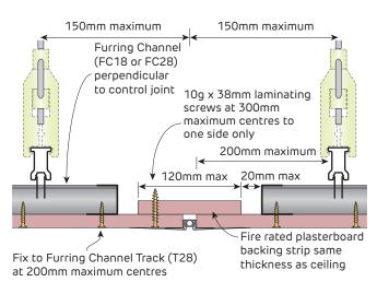
FIGURE 99 Seismic Control Joint Perpendicular to furring channel Section
