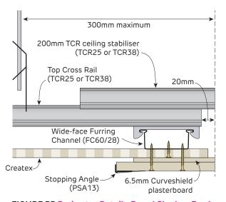
FIGURE 35 Perimeter Detail - Proud Shadow Border
