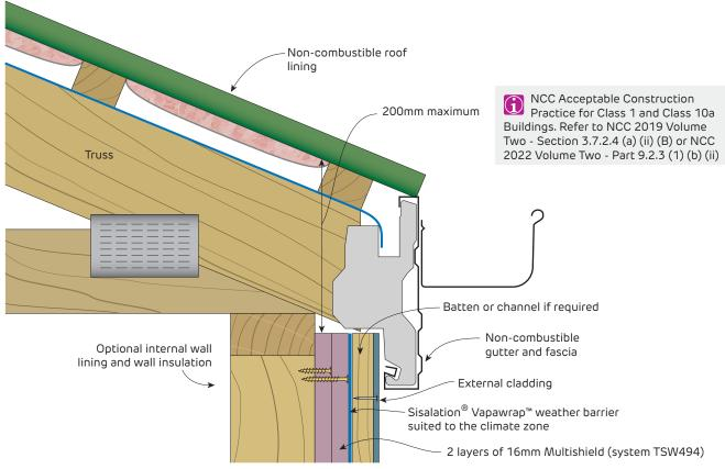
FIGURE 23 External Timber Wall to Non-combustible Gutter and Fascia
