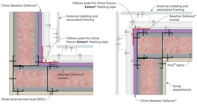
FIGURE 19 Exterior Internal Corner Plan
