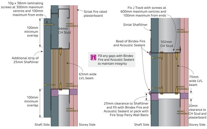
**FIGURE 42 Detail using LVL Beam with 64mm CH Studs** SHW2 Section
