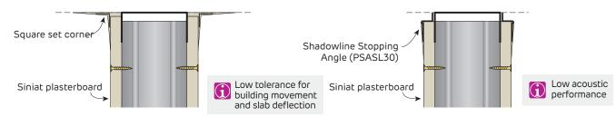
**FIGURE 53 Wall Head - Square Set** Section
