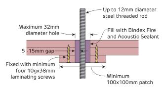
FIGURE 130 Up to 12mm steel diameter threaded rod Maintains RISF and FRL of ceiling under floor/roof systems Patch below ceiling lining Valid for 2 layers only - Section
