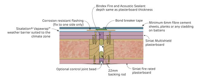
**FIGURE 33 Control Joint**
