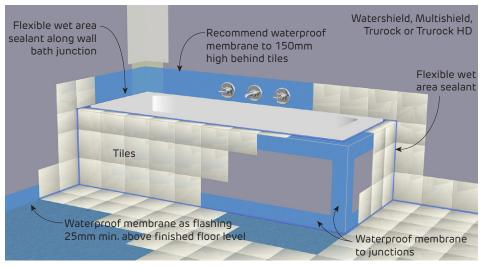
FIGURE 2 Bath (without shower) installation on timber flooring
