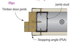
FIGURE 34 Typical Timber Door Jamb
