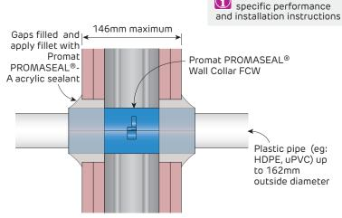
Refer to proprietary fire product manufacturer for performance and installation detail as well as approval for use in the selected building element
