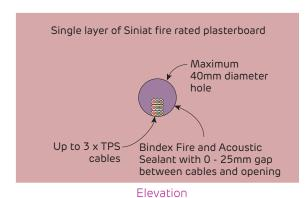
FRL requirements may be reduced to -/45/15 for penetrations in walls of Class 2 and 3 buildings not more than 25m in effective height. Refer to BCA Specification 18 for required conditions.
