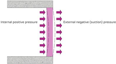
Enternal Wall  $C_{\rm shp,\,net} = C_{\rm shp,i} K_{\rm ci}$  acting with  $C_{\rm shp,e} K_{\rm ce}$
