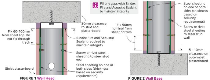
Steel sheeting between stud and plasterboard Section
