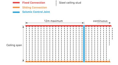
FIGURE 30 Stud Ceiling Type A1 - Fixed / Sliding
