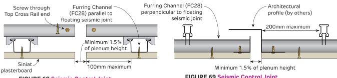
FIGURE 68 Seismic Control Joint
