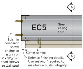
FIGURE 5 Fixed Connection EC5
