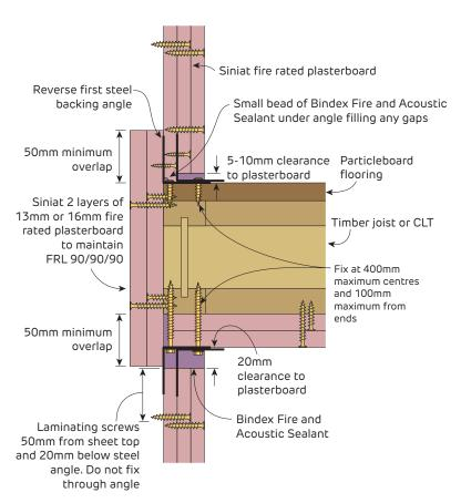
FIGURE 19 Laminated Vertical Shaft Around Fire Rated Timber Floor
