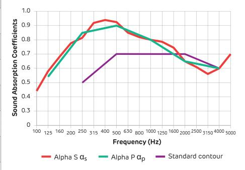
FIGURE 15 Sound Absorption Profile Comparing NRC with  $\alpha_{W}$
