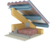
[Lateral restraint of truss bottom chord must be considered, ie: bottom chord ties and steelbrace]
