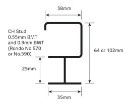
FIGURE 1 Shaft Wall CH Stud Section
