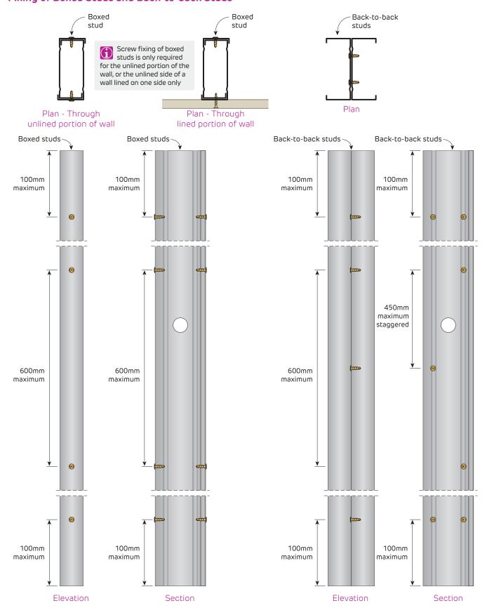
FIGURE 19 Fixing of Boxed Studs
