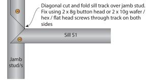
FIGURE 26b Sill S1 Connection 'cut and fold' Elevation
