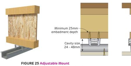
**FIGURE 25 Adjustable Mount**With 7mm holes suitable for Hex head screws Perspective and Sections
