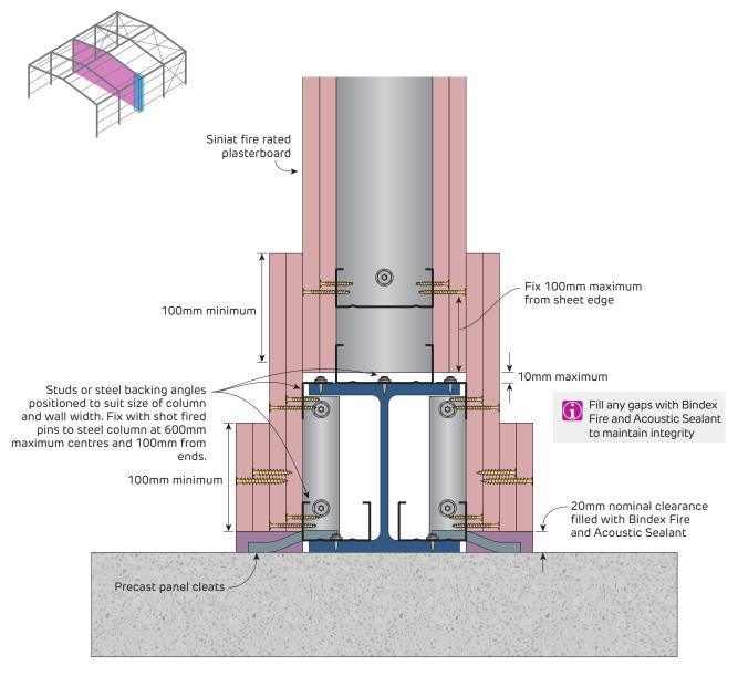
FIGURE 6 Wall End to Precast Wall
