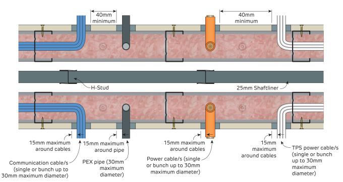
**FIGURE 49 Plumbing and Electrical Penetrations in Wall Linings** Plan
