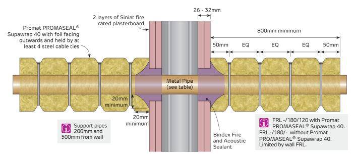
FIGURE 216 Metal Pipe Penetration wrapped with Supawrap 40
