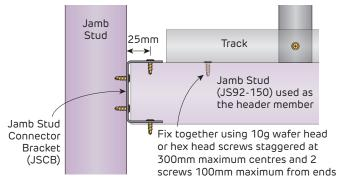
FIGURE 18b Header to Jamb Stud Connection for Prefabricated Door Frames Elevation
