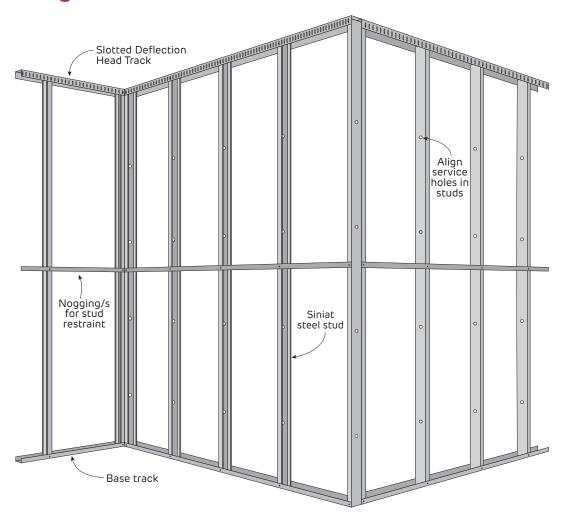
FIGURE 8 Typical External Steel Frame Wall Layout
