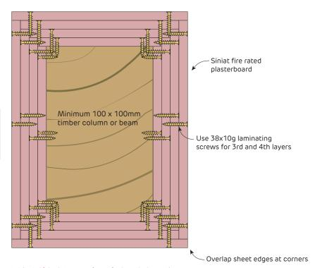
For corner gaps up to 3mm, fill with either Bindex Fire and Acoustic sealant or Mastabase jointing compound. Fill any other gaps with Bindex sealant to maintain integrity.
