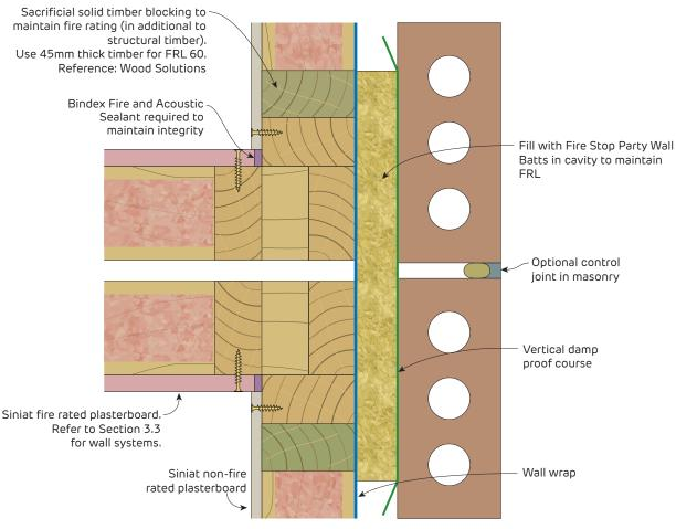
FIGURE 13 Separating Wall to External Brick Wall
