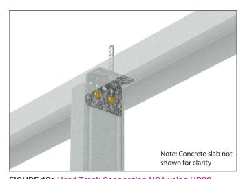
**FIGURE 18a Head Track Connection HC4 using UB80** Heavy Duty Connection for 92mm and 150mm studs Perspective
