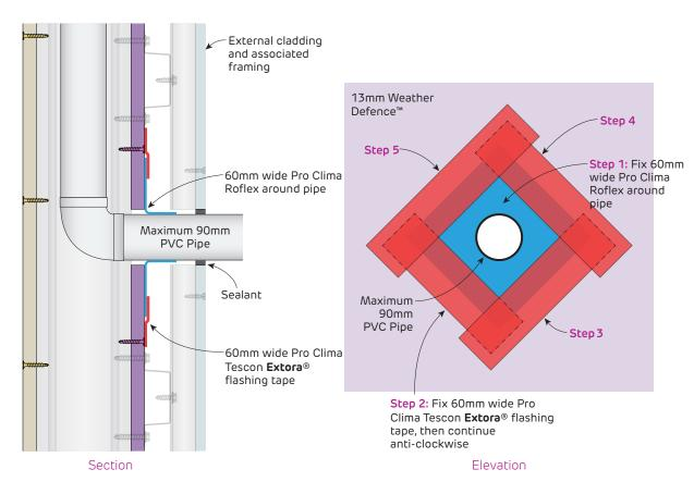
FIGURE 40 Drainage Outlet Detail
