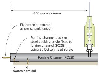
FIGURE 64 Furring Channel Fixed Connection
