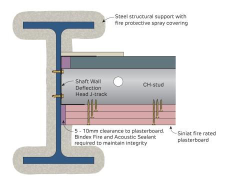
**FIGURE 9 Shaft Wall Ceiling to Structural Beam** Section
