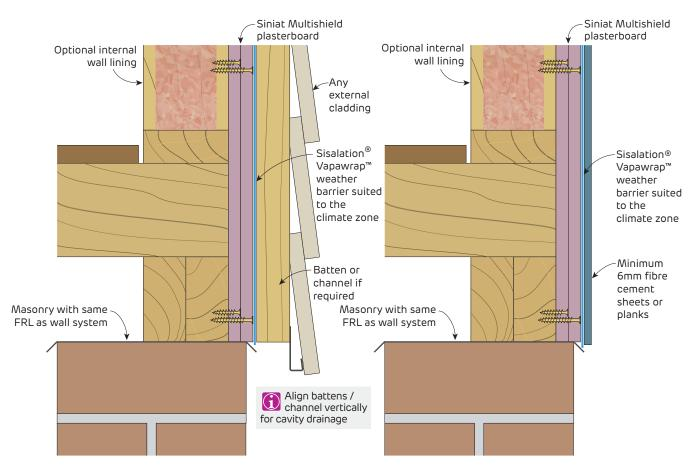
FIGURE 6 External Timber Wall Base with Sub-floor
