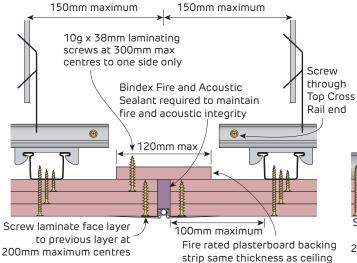
**FIGURE 102 Seismic Control Joint**
