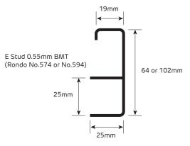
FIGURE 2 Shaft Wall E Stud Section
