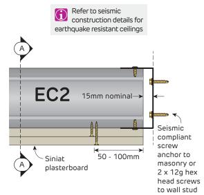
FIGURE 6 Sliding Connection EC2 Slotted Deflection Head Track Section
