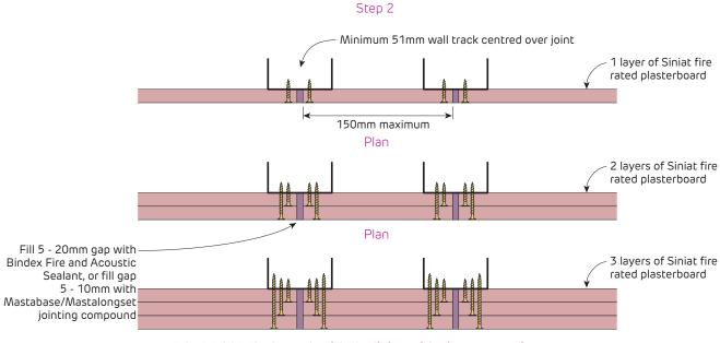
**FIGURE 217 Flush patch with the lining with pipe penetration**Maximum 150mm pipes as per Table 19 - Refer to previous pages for FRL
