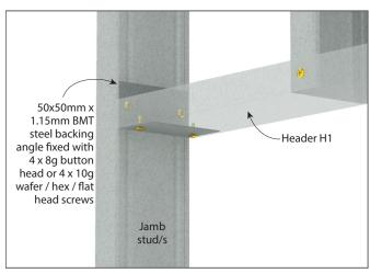
FIGURE 24a Alternative Header H1 Connection 'A-2' Perspective
