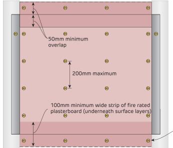
Install backing strips of fire rated plasterboard and fix using 10g x 38mm laminating screws at 200mm maximum
