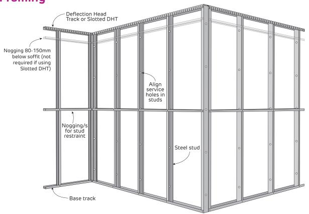
FIGURE 1 Typical External Steel Frame Wall Layout
