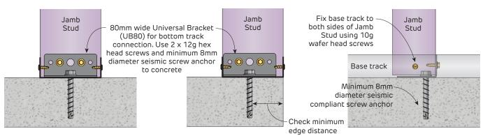
FIGURE 25a Base Connection BC6 for Door Opening
