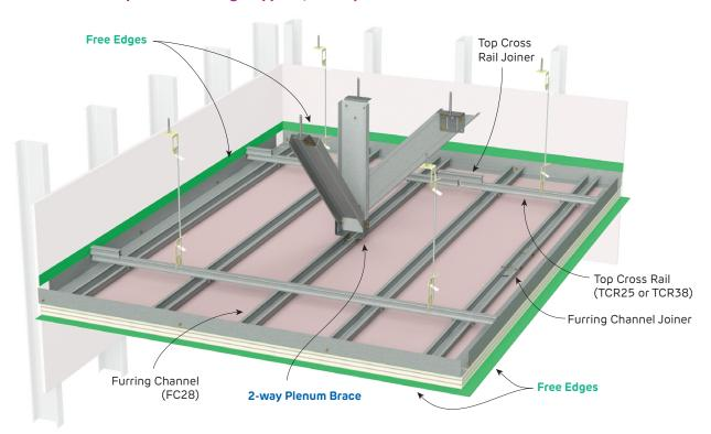
FIGURE 77 Suspended Ceiling Frame - Type C, 2-way Plenum Braced 2-way Plenum Brace with four sides Free
