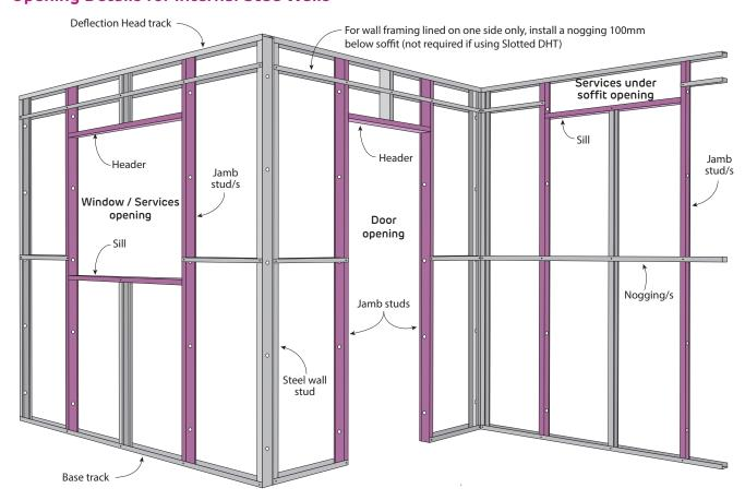
FIGURE 1 Internal Steel Frame Wall with Window and Door Openings
