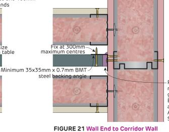
Fill 20mm maximum gap with Bindex Fire and Acoustic Sealant
