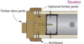
FIGURE 30 Typical Timber Door Jamb Plan
