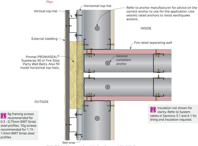
FIGURE 116 Internal Stud Wall to External Clad Wall
