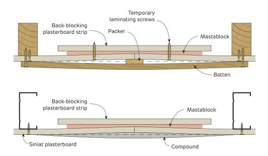
FIGURE 5 Creating a Recess on a Wall Butt Joint using a Temporary Packer  $\mathsf{Plan}$
