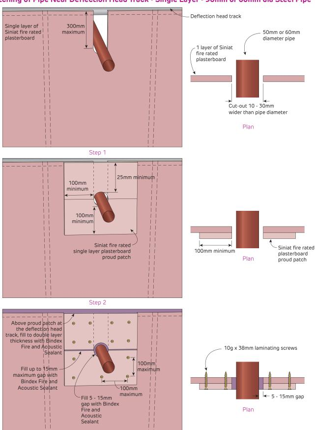
Step 3 **FIGURE 219 Proud patch around steel pipe penetration near deflection head track**Maximum 60mm diameter pipe - FRL -/60/30
