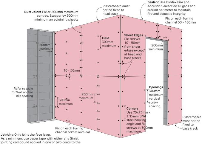
jointing compound applied in one or two coats to the thickness of two coats. Alternatively, for butt joints only, use Bindex Fire and Acoustic Sealant according to the Product Data Sheet.
