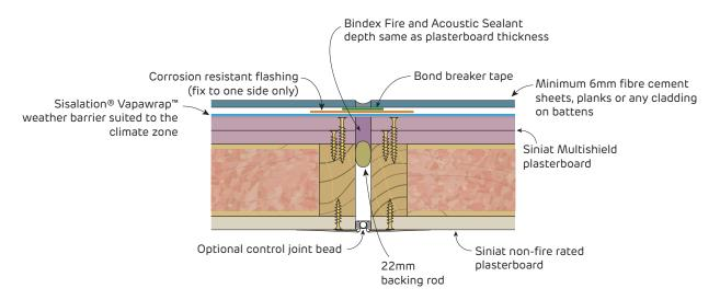
**FIGURE 32 Control Joint**
