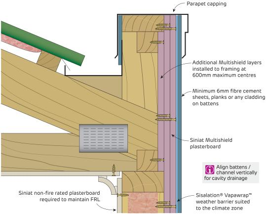
FIGURE 24 External Timber Wall to Non-combustible Roof Lining
