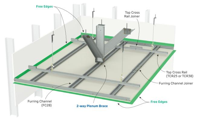
FIGURE 76 Suspended Ceiling - Type C, 2-way Plenum Braced 2-way Plenum Brace with four sides Free Perspective
