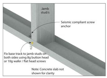
FIGURE 20a Base Track Connection BC3 - Window Perspective
