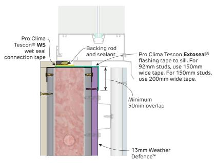
FIGURE 35 Window Sill Detail
