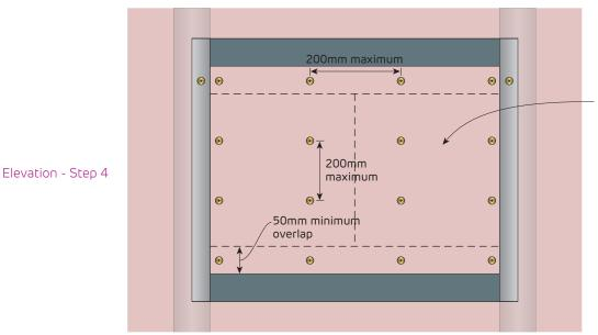
Install cover strip of fire rated plasterboard over Shaftliner Panel and fix using 10g x 38mm laminating screws at 200x200mm maximum
