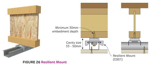
With 6.5mm hole suitable for Hex head screws Perspective and Sections
