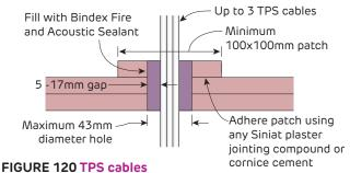
Maintains FRL of ceiling under floor/roof systems Patch above ceiling lining Valid for 2 layers only - Section
