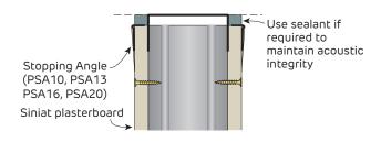
FIGURE 51 Wall Head - Stopping Angle Section
