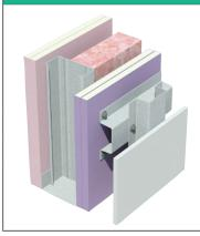
2 layers of 13mm fireshield or multishield or impactshield or trurock
