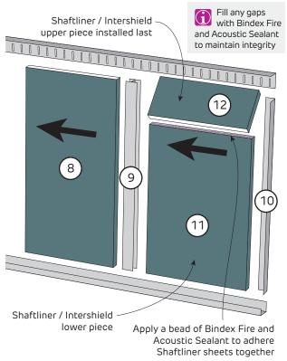
FIGURE 7 Alternative Shaftliner End Construction Step 1 - Perspective
