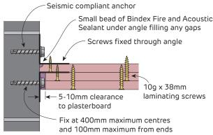
**FIGURE 7 Laminated Vertical Shaft to Masonry Wall** Plan view
