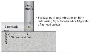
FIGURE 19c Base Track Connection BC3 for Door Opening Elevation
