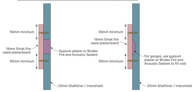
FIGURE 75 Fire Rated Patch for Shaftliner panel
