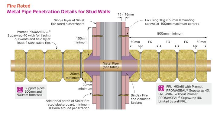
FIGURE 215 Metal Pipe Penetration wrapped with Supawrap 40
