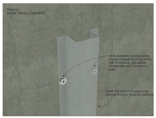
**FIGURE 6 Top Hat over Masonry Wall**Vertical or Horizontal Top Hats directly fixed to masonry Perspective
