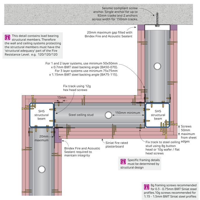
FIGURE 69 Stud Wall with Integrated Bulkhead Section
