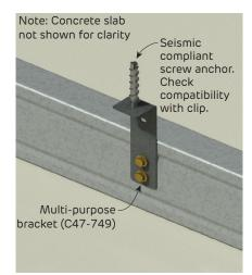
**FIGURE 43 Multi-purpose Bracket**Option 1 Light Duty Connection
