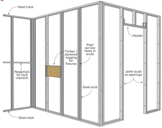
FIGURE 1 Internal Steel Frame Wall Layout
