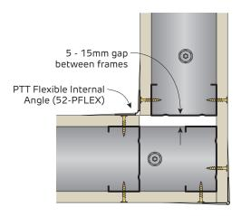
FIGURE 66 Sliding Wall Corner Plan
