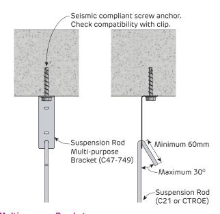
FIGURE 29 Suspension Rod Multi-purpose Bracket
