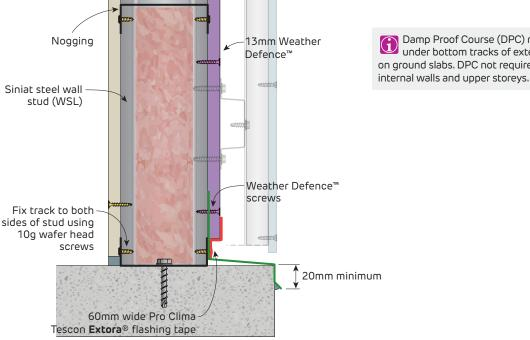
FIGURE 25 Wall Base to Concrete Slab Section
