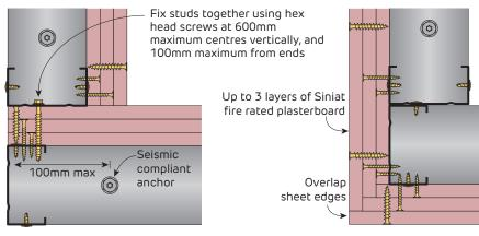
FIGURE 108 90° Internal Corner Plan
