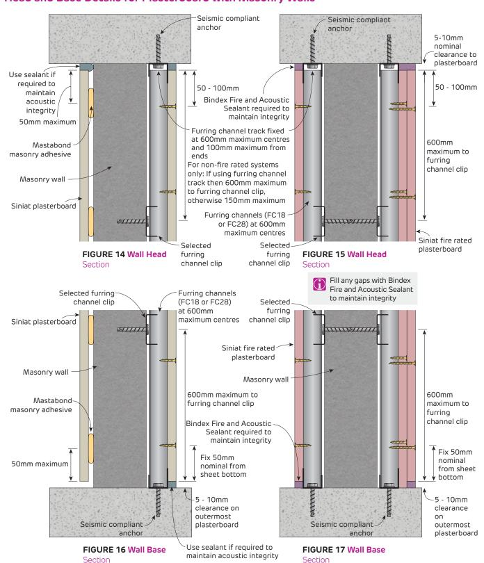
Outermost plasterboard sheets with no gap at the base are at risk of moisture wicking
