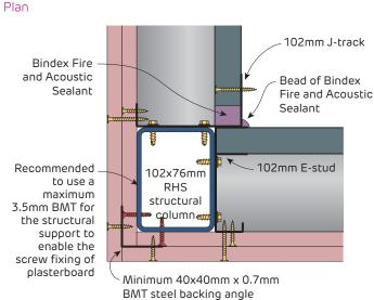
FIGURE 24 Shaft Wall Bulkhead External Corner using RHS Column with 102mm CH-Studs SHW2 Plan
