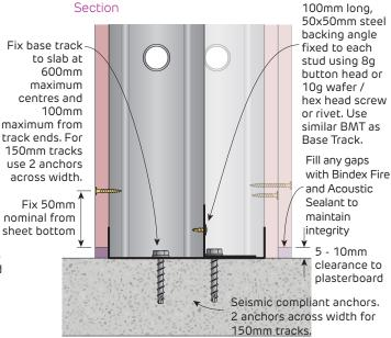
FIGURE 127 Wall Base - Staggered Stud 92mm Studs in 150mm Base Track Section
