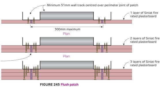
Fill 5 - 20mm gap with Bindex Fire and Acoustic Sealant, or fill gap 5 - 10mm with Mastabase/Mastalongs et jointing compound and allow to set. Then set the joint in the normal fashion using paper tape with any Siniat jointing compound.
