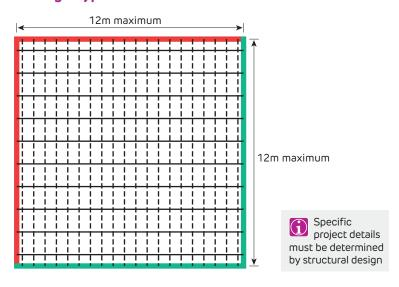
FIGURE 62 Suspended Ceiling - Type B1
