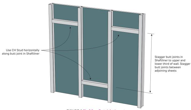
FIGURE 6 Shaftliner Butt Joint Layout
