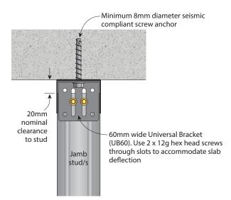
**FIGURE 17b Head Track Connection HC4**Heavy Duty Connection for 64mm and 76mm studs
