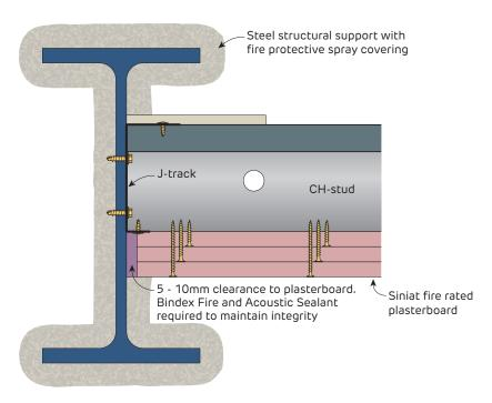
**FIGURE 8 Shaft Wall Ceiling to Structural Beam** Section
