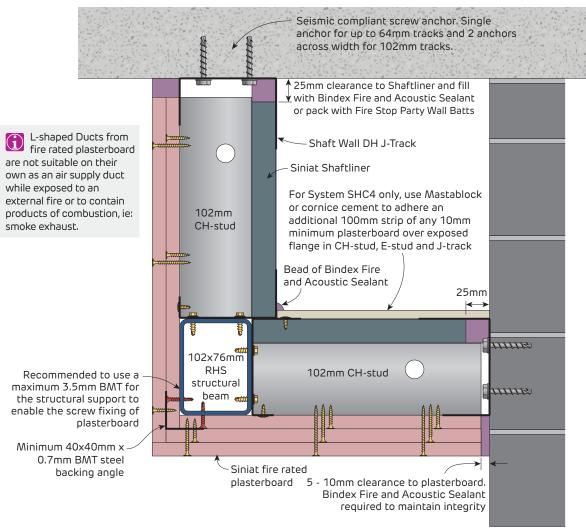
**FIGURE 11 Shaft Wall L-shaped Duct with RHS Structural Beam** SHW2 and SHC4 Section
