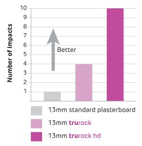
FIGURE 20 Large Hard Body Impact Testing
