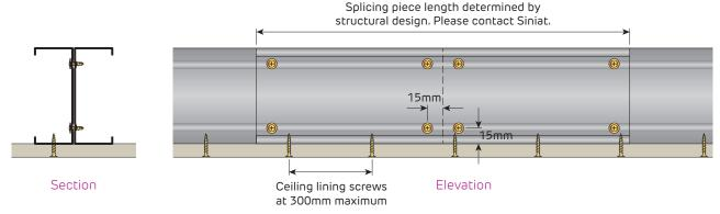
FIGURE 59 Splicing Steel Ceiling Studs via Back-to-back Method
