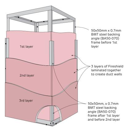
FIGURE 1 Framing and Plasterboard Layout
