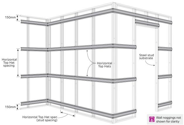
FIGURE 2 Horizontal Steel Top Hat Layout
