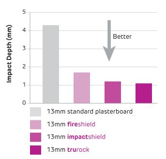
FIGURE 21 Small Hard Body Impact Testing
