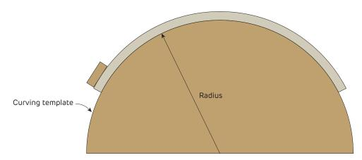
**FIGURE 19 Curving Template** Section
