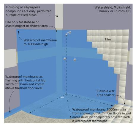
FIGURE 3 Internal in situ tray for unenclosed shower
