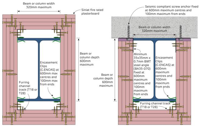
FIGURE 4 4 Sided Protection for I-Beam/Column Plan or Section
