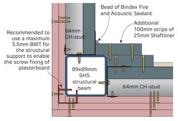
FIGURE 16 Alternative Detail using SHS Beam with 64mm CH-Studs
