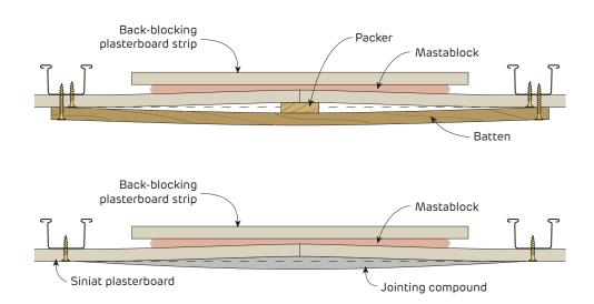
FIGURE 4 Creating a Recess on a Ceiling Butt Joint using a Temporary Packer Section
