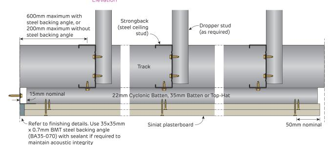
**SECTION N-N Ceiling Edge** Section **SECTION N-N Ceiling Stud Detail** Section
