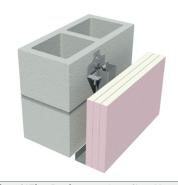
This system is designed to upgrade the FRL of the masonry wall
