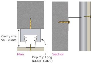
**FIGURE 11 Grip Clip Long**With 6.5mm hole suitable for Hex head screws
