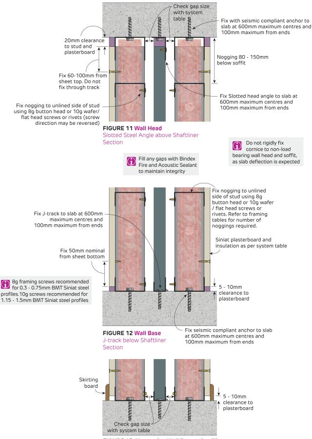
FIGURE 13 Alternative Wall Base using Rivets
