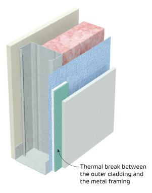
**FIGURE 17 Installation of Thermal Break**Perspective
