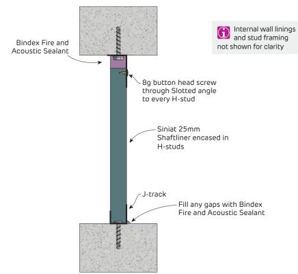
FIGURE 10 Central Fire Barrier Section
