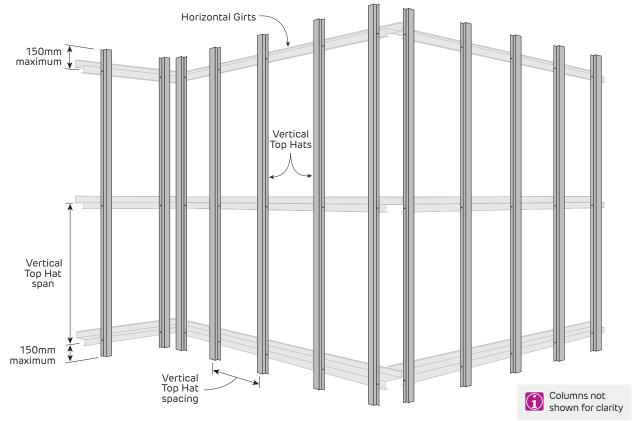
FIGURE 1 Vertical Steel Top Hat Layout
