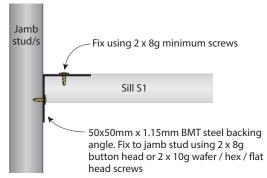
FIGURE 27b Alternative Sill S1 Connection 'A-2' Elevation
