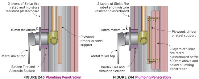
FIGURE 243 Plumbing Penetration
