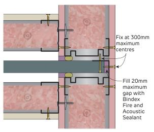
FIGURE 23 Wall End to Corridor Wall Improved Acoustic Detail - Steel angle Plan
