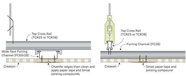
FIGURE 20 Butt Joints Section
