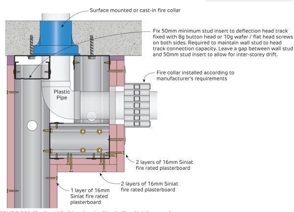
FIGURE 229 Fire Rated Bulkhead under Plastic Pipe Slab Penetration
