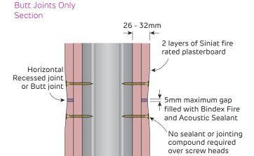
FIGURE 233 Horizontal Joints in Double Layer Wall Systems
