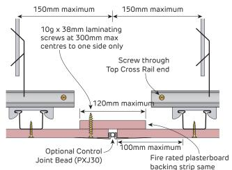
FIGURE 98 Seismic Control Joint thickness as ceiling Parallel to furring channel Section
