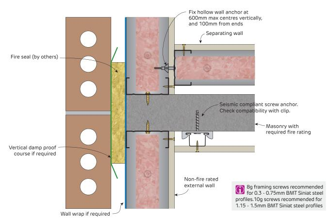
**FIGURE 27 Typical Internal Masonry Separating Wall to Brick Veneer** Example Only
