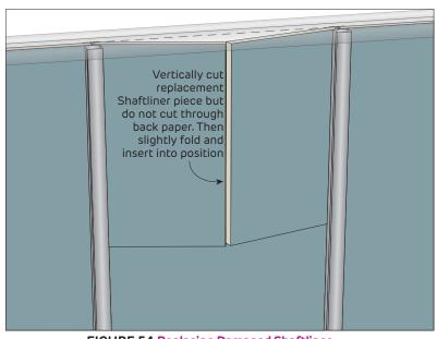
FIGURE 54 Replacing Damaged Shaftliner
