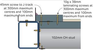
FIGURE 13 Construction of Shaft Wall Ceiling and Bulkhead Section
