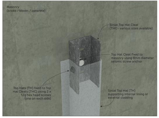
**FIGURE 5 Top Hat Cleat over Masonry Wall**Vertical or Horizontal Top Hats over Top Hat Cleats
