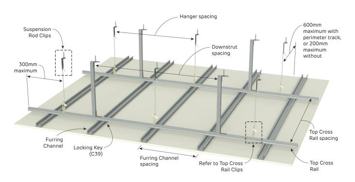
**FIGURE 6 Suspended Ceiling Frame with Downstruts**Perspective
