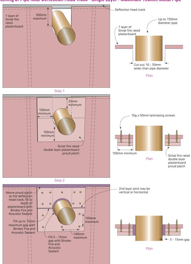
Step 3 FIGURE 220 Proud patch around metal pipe penetration near deflection head track
