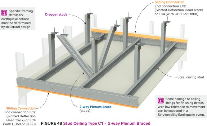
FIGURE 48 Stud Ceiling Type C1 - 2-way Plenum Braced Perspective
