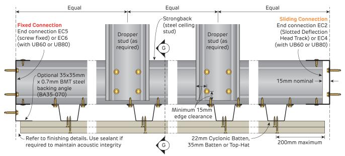
FIGURE 39 Stud Ceiling Type A3 - Fixed / Sliding Flevation
