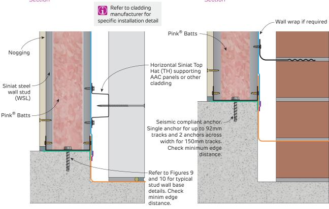
**FIGURE 24 External Steel Stud Wall Base**With horizontal Top Hats under AAC
