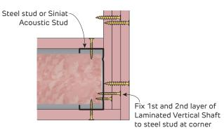
FIGURE 17 Laminated Vertical Shaft Corner Transition to Steel Framed Partition Wall Plan view
