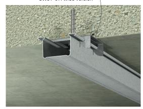
**FIGURE 4 Anchor Clip and Furring Channel** Perspective
