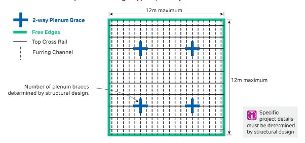
FIGURE 78 Suspended Ceiling - Type C, 2-way Plenum Braced 2-way Plenum Brace with four sides Free Plan
