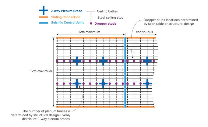
FIGURE 53 Stud Ceiling Type C2 - 2-way Plenum Braced Plan
