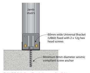
**FIGURE 21b BaseTrack Connection BC4**Heavy Duty Connection for 64mm and 76mm studs
