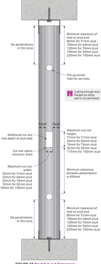
FIGURE 21 Stud Cut-out Tolerances
