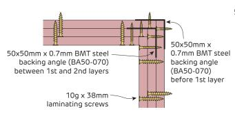
FIGURE 9 Laminated Vertical Shaft Internal Corner
