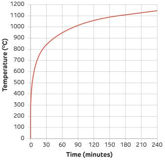
**FIGURE 12 Standard Fire Test** Time - Temperature curve
