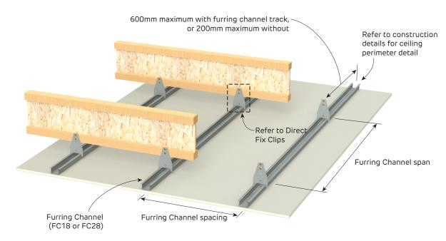
**FIGURE 1 Direct Fix Furring Channel Ceiling Frame**Perspective
