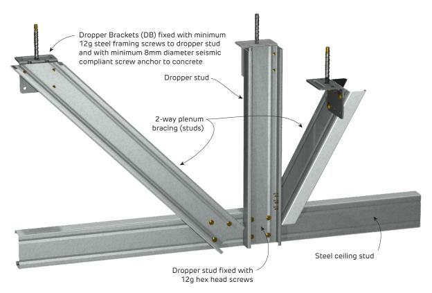
FIGURE 56 2-way Plenum Brace Perspective
