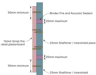
FIGURE 76 Fire Rated Patch for Shaftliner panel
