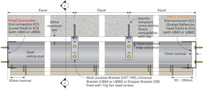
FIGURE 46 Stud Ceiling Type A4 - Fixed / Sliding Elevation
