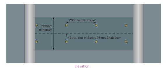
**FIGURE 17 Butt Joint in Shaftliner** Section
