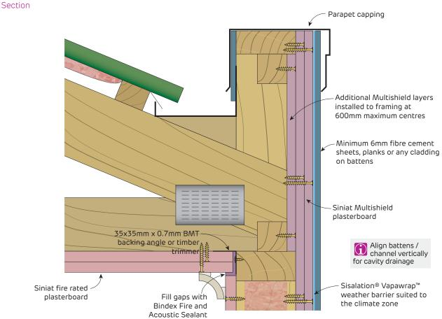
FIGURE 25 External Timber Wall to Non-combustible Roof Lining
