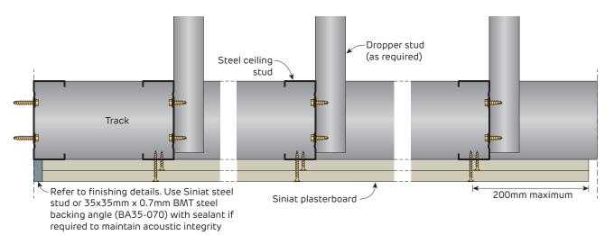
**SECTION L-L Ceiling Edge** Section
