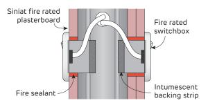
Refer to proprietary fire product manufacturer for performance and specific installation detail as well as approval for use in the selected building element.
