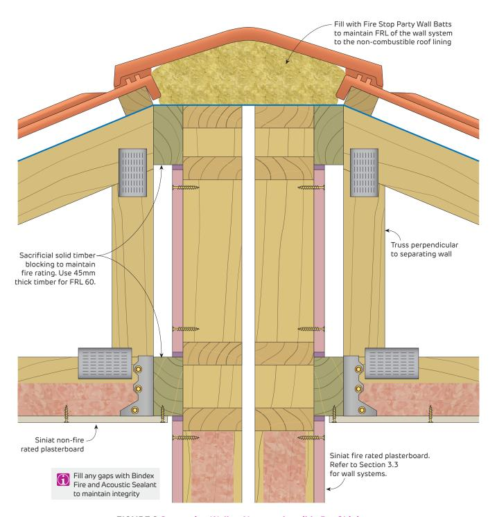
FIGURE 9 Separating Wall to Non-combustible Roof Lining FRL 60/60/60 Section
