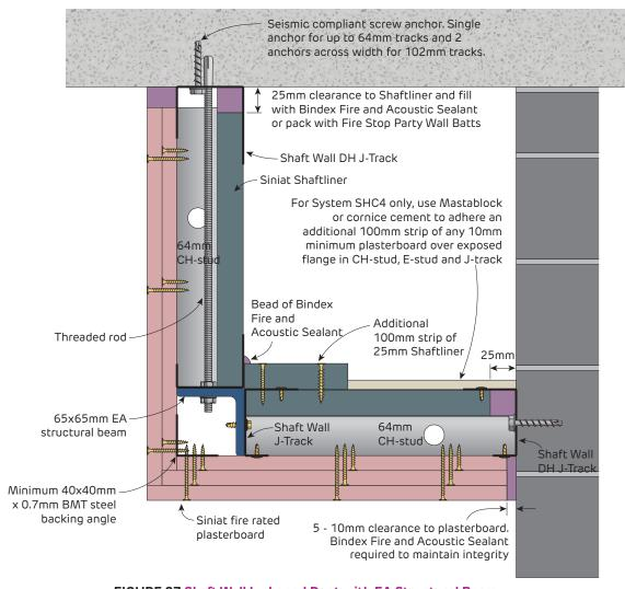
FIGURE 27 Shaft Wall L-shaped Duct with EA Structural Beam SHW2 and SHC4 Section
