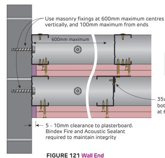
Set the face layer of both sets of fire rated plasterboard layers
