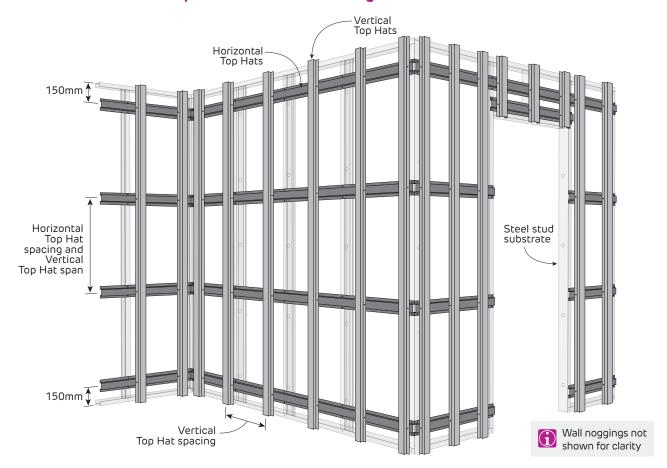
FIGURE 3 Vertical Top Hats over Horizontal Top Hats
