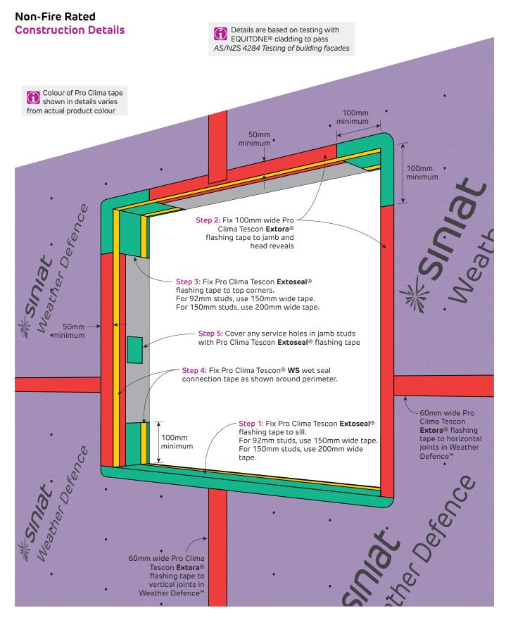
**FIGURE 32 Flashing Tapes Around Openings**Perspective
