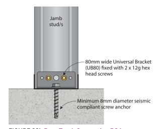
**FIGURE 22b Base Track Connection BC4**Heavy Duty Connection for 92mm and 150mm studs Section
