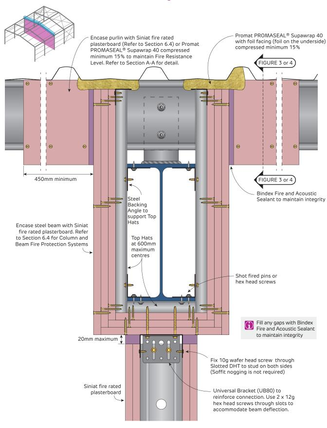
FIGURE 1 Wall Head Detail Up to FRL 120/120/120
