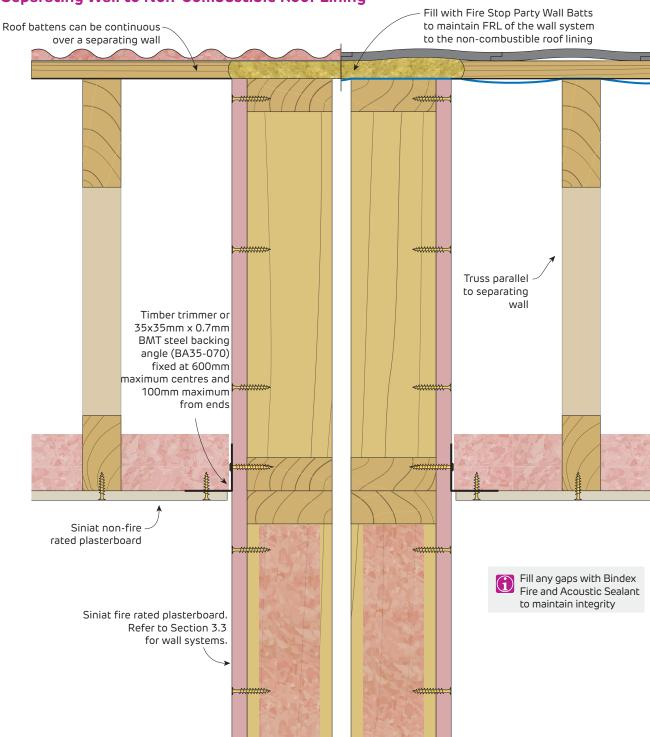
FIGURE 8 Separating Wall to Non-combustible Roof Lining  $\mbox{FRL}\,60/60/60$
