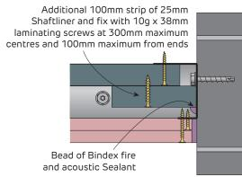
Fill any gaps with Bindex Fire and Acoustic Sealant to maintain integrity FIGURE 21 Alternative Shaft Wall End
