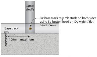
FIGURE 20b Base Connection BC3 for Window Opening Elevation
