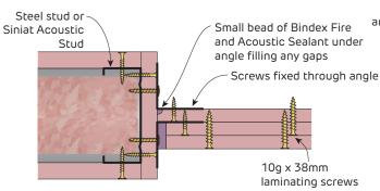
FIGURE 15 Laminated Vertical Shaft Transition to Steel Framed Partition Wall
