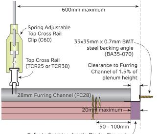
Refer to finishing details. Bindex Fire and Acoutic Sealant required to maintain inegrity
