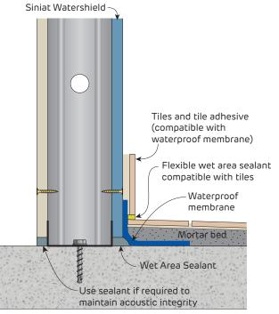
**FIGURE 14 Wall Base in General Wet Area**Outside shower - Class 3 membrane shown
