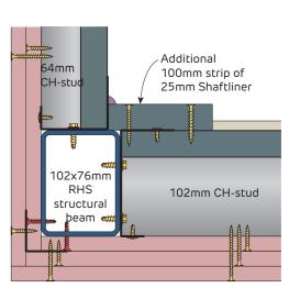
FIGURE 12 Alternative detail using RHS Beam with 64 and 102mm CH-Studs SHW2 and SHC4 Section
