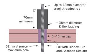
FIGURE 134 Up to 12mm steel diameter threaded rod Maintains RISF and FRL of Universal Ceiling Systems Valid for 3 to 4 layers only Section
