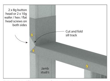
FIGURE 26a Sill S1 Connection 'cut and fold'
