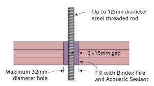
FIGURE 131 Up to 12mm steel diameter threaded rod Maintains RISF and FRL of ceiling under floor/roof systems Valid for 3 layers only Section
