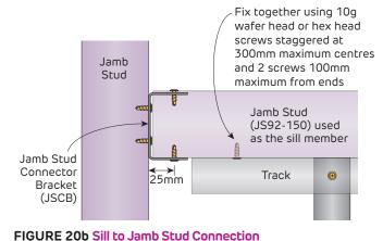
With Jamb Stud Connector Bracket Elevation
