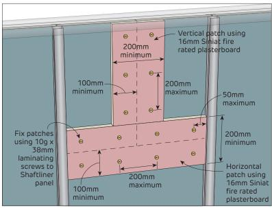
**FIGURE 54 continued Replacing Damaged Shaftliner**Perspective
